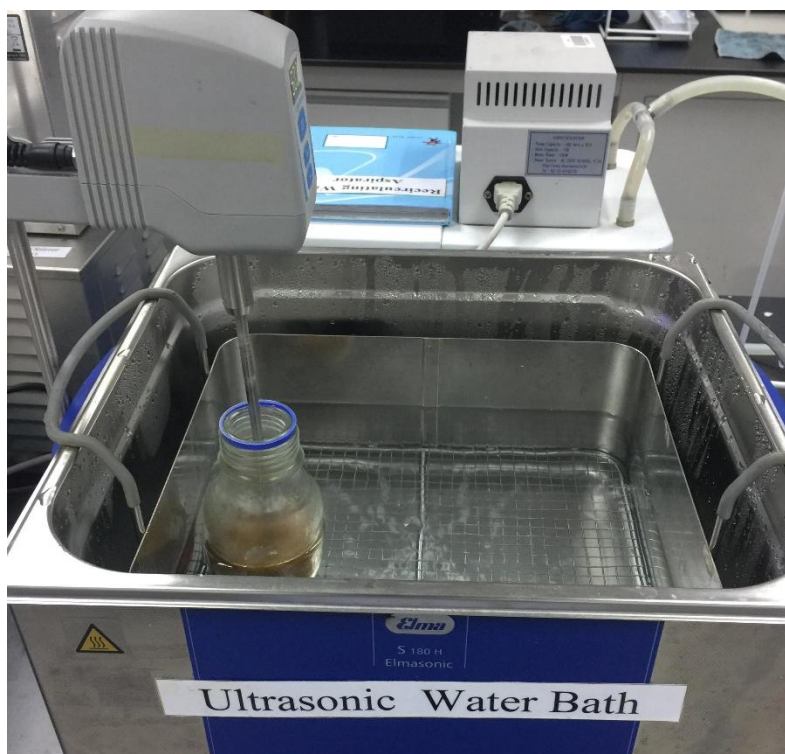
Figure 3.2: Set-up of Treatment with NaOH in an Ultrasonic Water Bath
