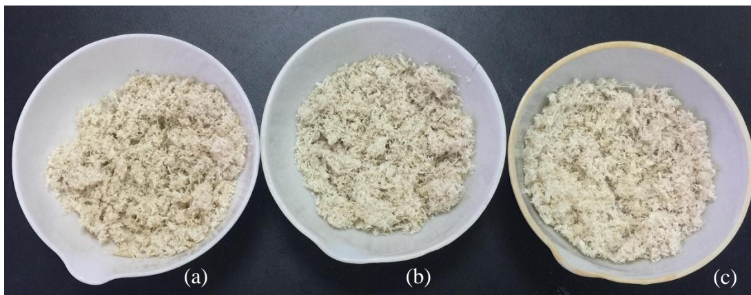
Figure 4.6: Appearance of Treated SCB after Treatment at Various Temperature of (a) 60 °C (b) 70 °C (c) 80 °C
