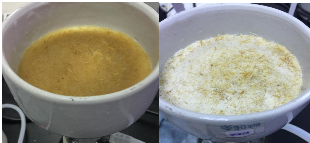
Figure 4.5: Treated SCB Before and After Washing with Distilled Water and Hot Ethanol
