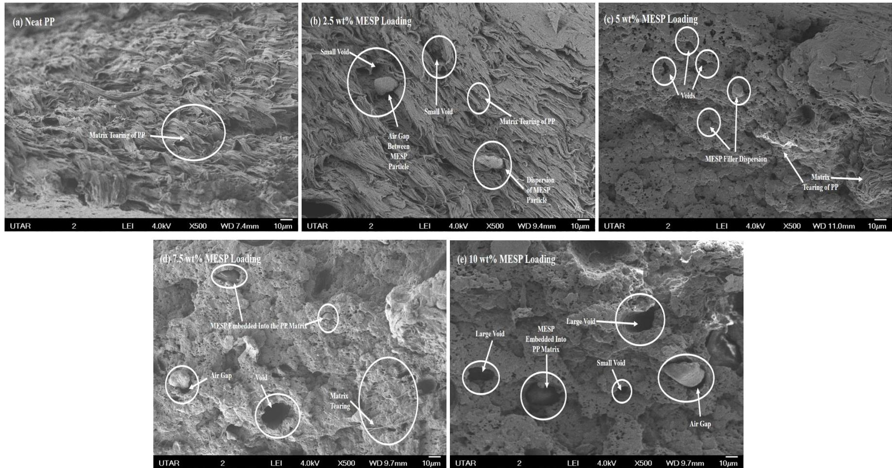
Figure 4.10: Comparison of Tensile Fractured Surface Morphology of PP/MESP Composites; (a) Neat PP, (b) PP/MESP -2.5 %, (c) PP/MESP -5.0 %, (d) PP/MESP -7.5 %, (e) PP/MESP -10.0 % at 500x Magnification.
