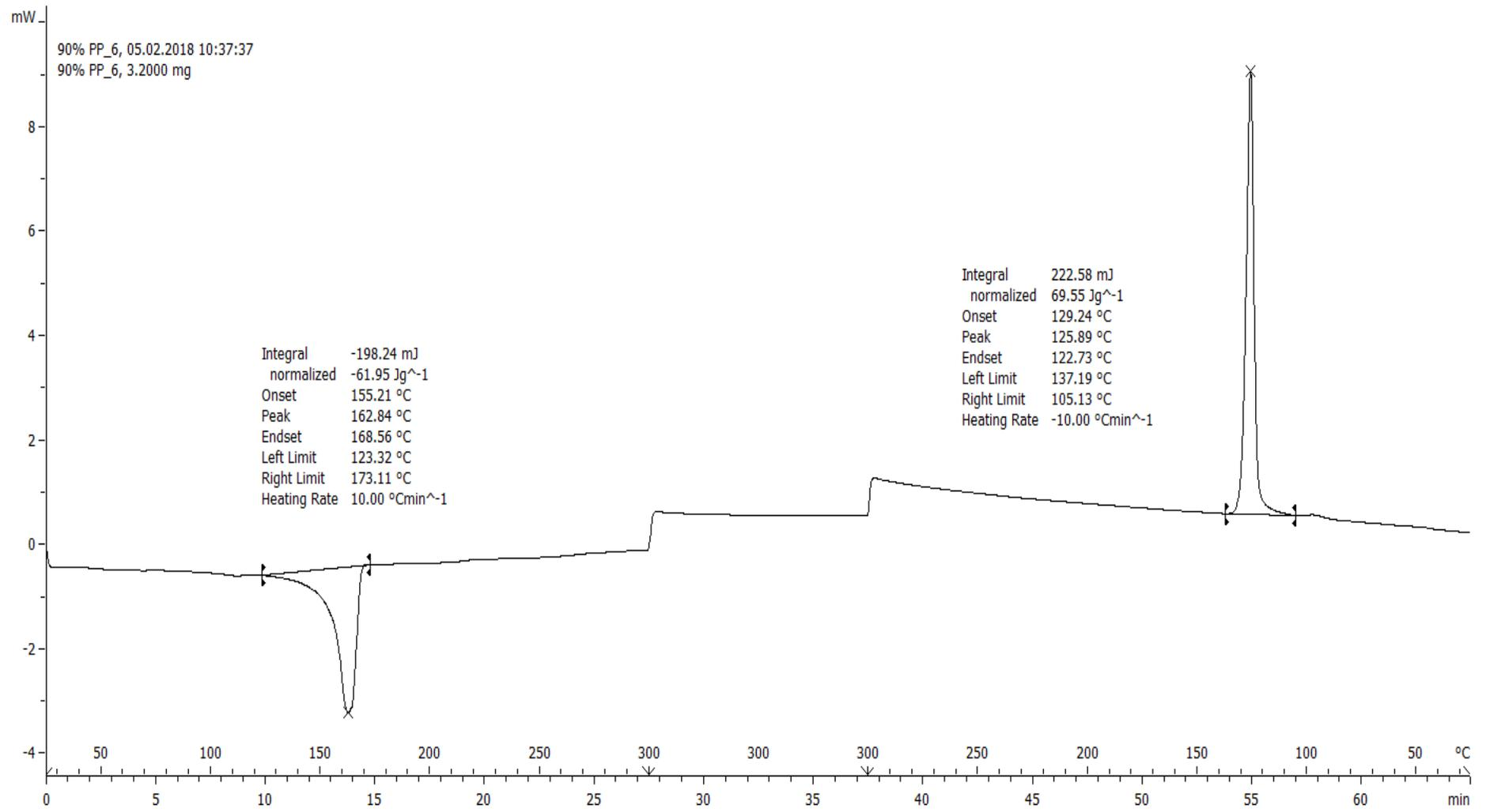
(f) Crystallization Curve of PP/MESP Composites at Different Loadings
