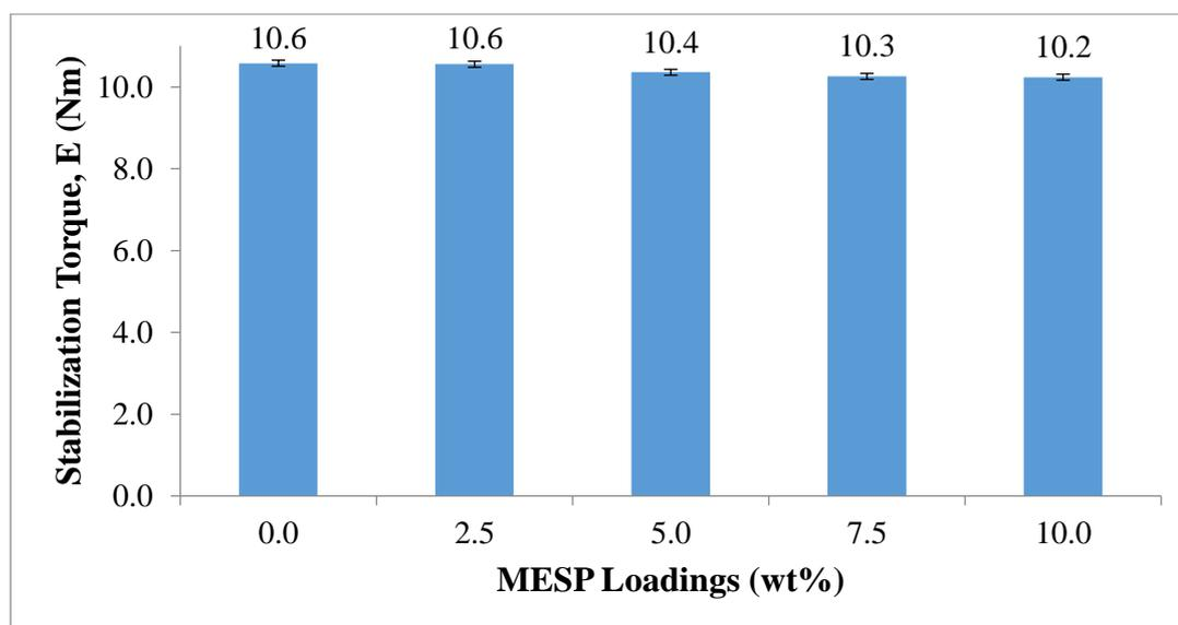
Figure 4.6: Stabilization Torque of PP/MESP Composites at Different MESP Loadings.
