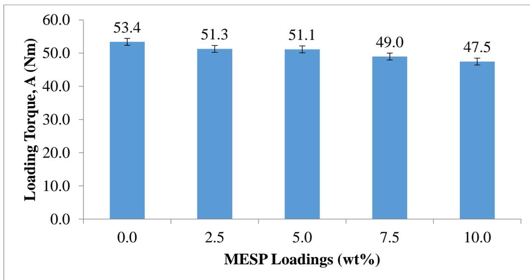
Figure 4.5: Loading Torque of PP/MESP Composites at Different MESP Loadings.
