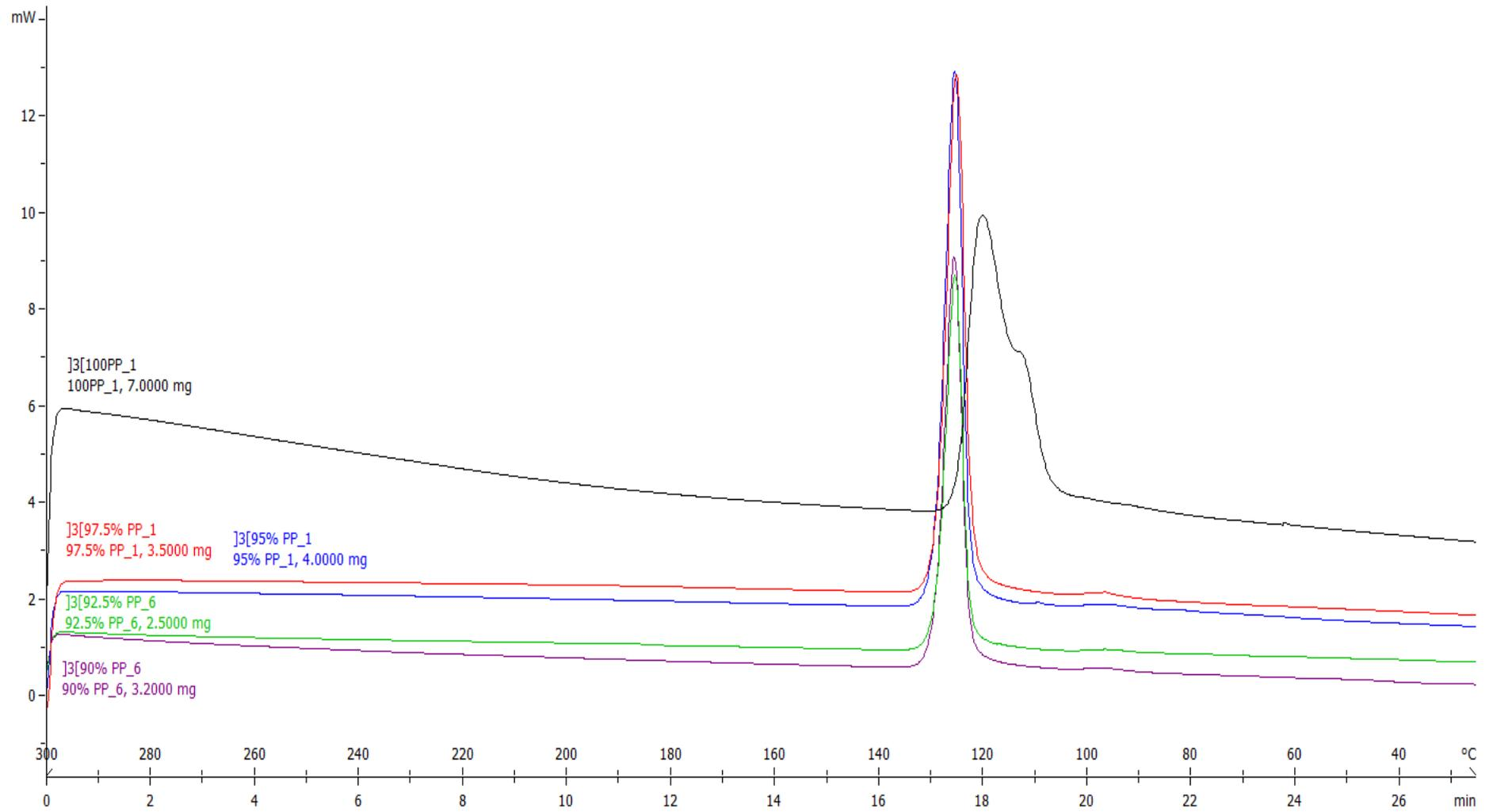
(g) Melting Curve of PP/MESP Composites at Different Loadings
