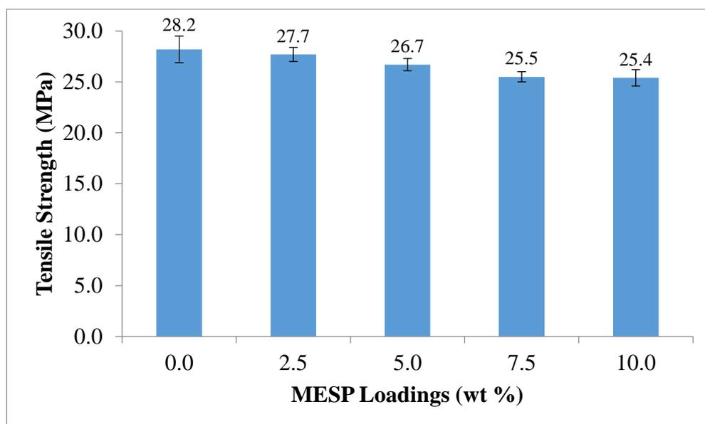
Figure 4.7: Variation in Tensile Strength of PP/MESP Composites.
