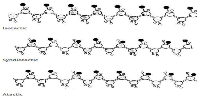
Figure 2.1: Different Molecular Configurations of Polypropylene (Michieal, 2015).
