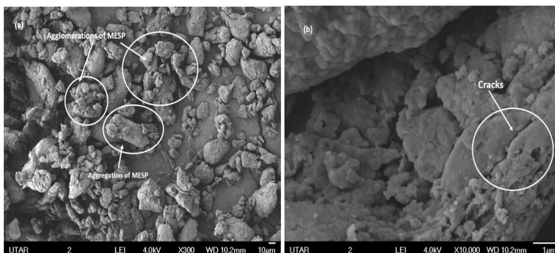
Figure 4.3: Micrograph of MESP particles surface at (a) 300x Magnification (b) 10,000x Magnification
