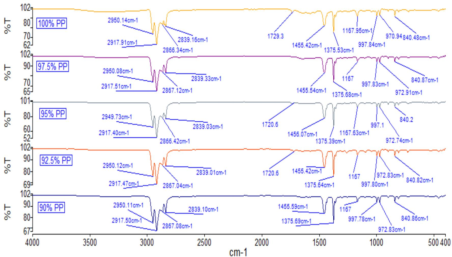
Figure 4.4: FTIR-ATR Spectra of PP/MESP Composites at Different MESP Loadings.
