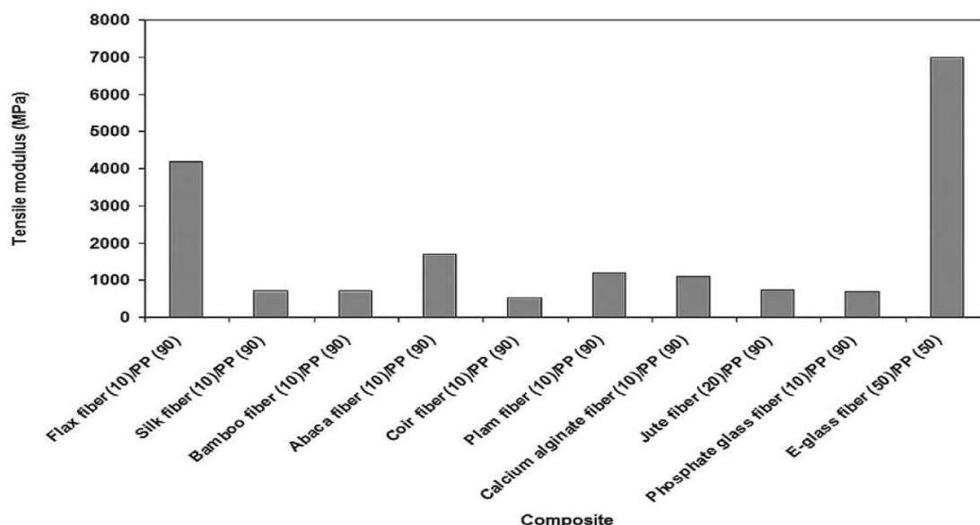
Figure 2.7: Tensile Modulus of Different Fibre-Reinforced PP Composites (FRPCs), (Quaiyyum, et al., 2011).
