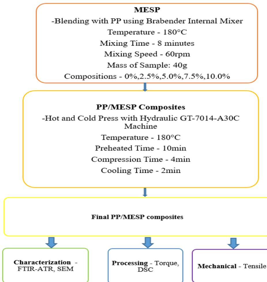
Figure 3.4: Flowchart of Preparation and Testing of PP/MESP Composites.
