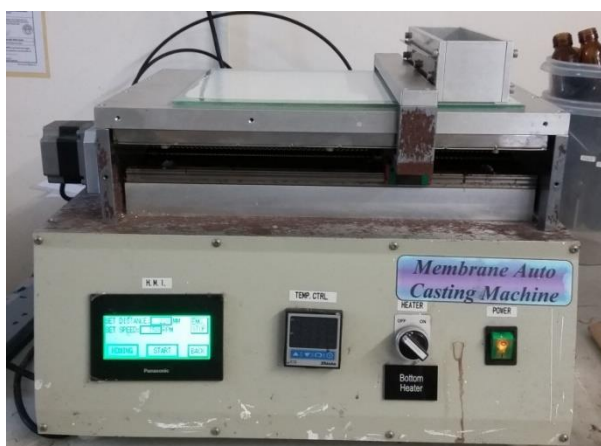
Figure 3.4: Membrane Auto Casting Machine Setup.
