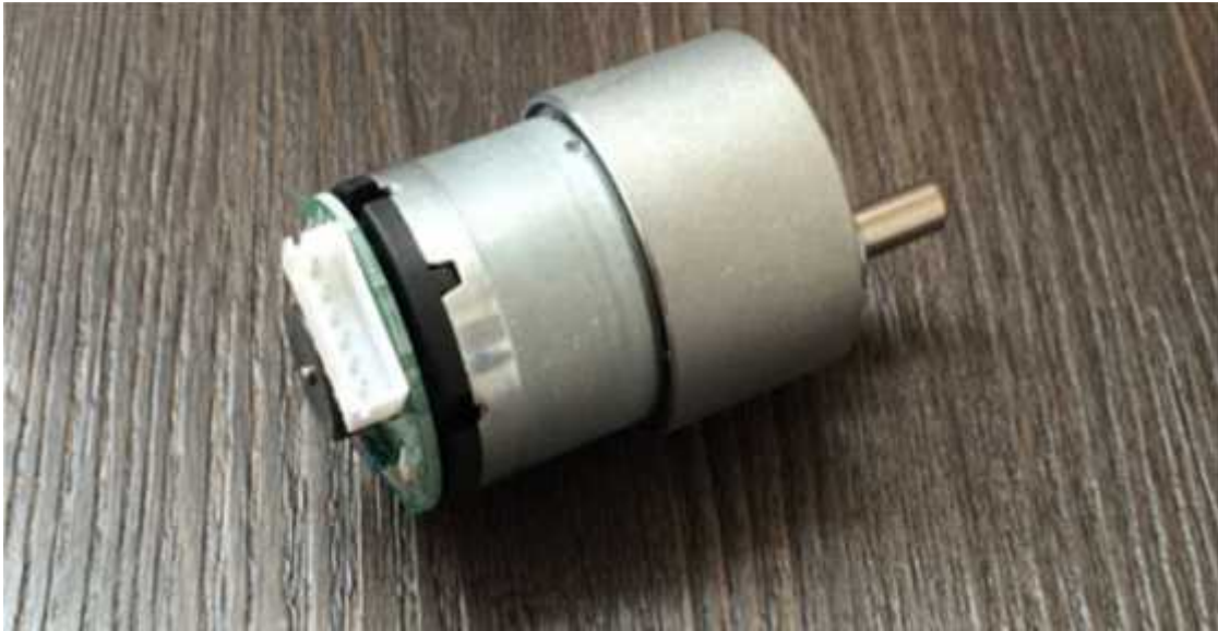
Figure 4-2-6 DC gear motor mounted quadrature encoder
