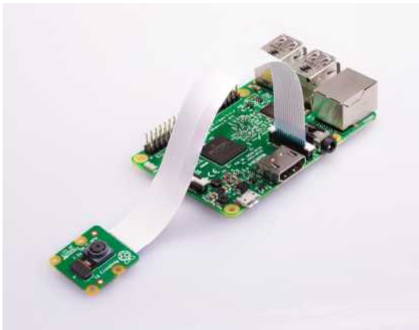
Figure 3-7-13 Connection of Raspberry Pi 2 Model B and Pi Camera
