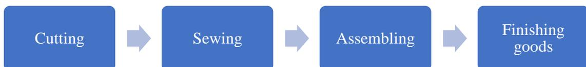
After receives of raw material from the inbound area, production labor will measure and cut the material for the following production. Next, they will sew the compartment pocket and velcro straps. Further on, labor in the assembly stage need to combine the entire product and place in the water bladder. Lastly, finishing good will send to the labeling and packaging area to wrap up.
