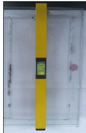
The glass plate was ensured to be flat by using the water level ruler.
