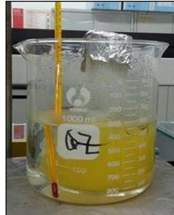
Different weight ratio of CPWF was added to the clear PVA solution with continuously stirring for about one and a half hour.
