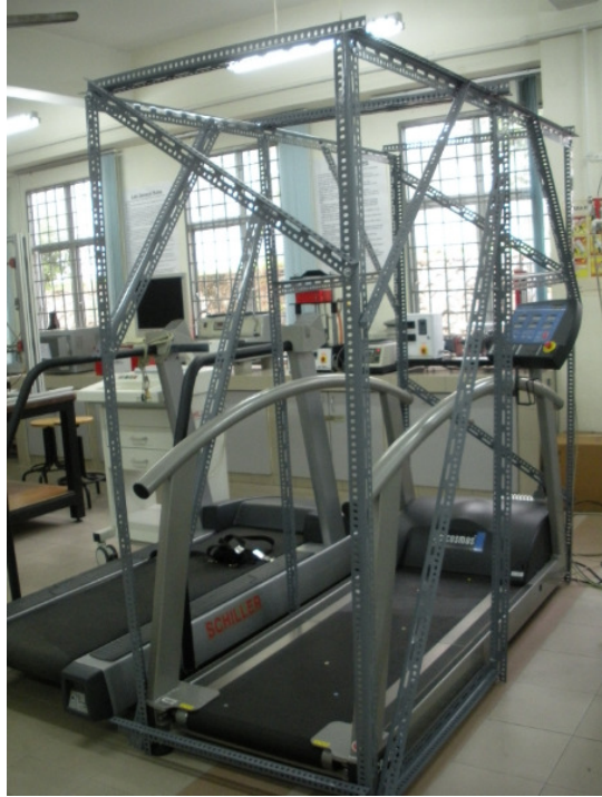
Figure 3.10: Supporting structure to place the safety belt
