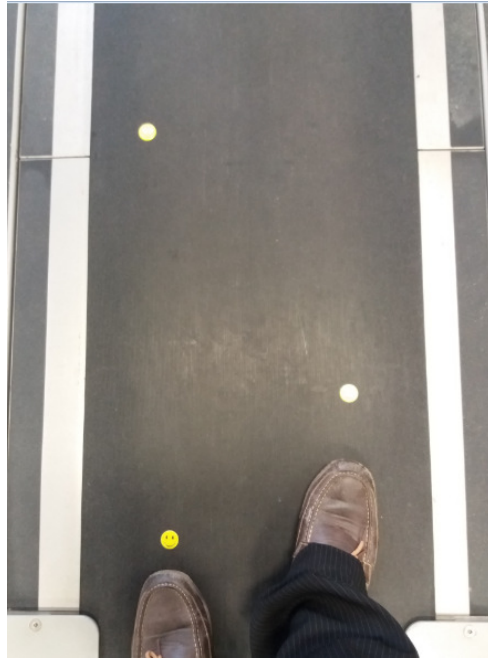
Figure 3.13: Subject need to avoid stepping on randomly pasted round stickers to simulate abnormal gaits
