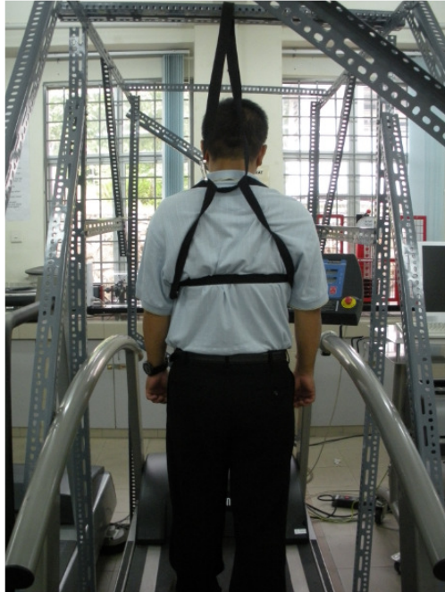
Figure 3.14: The safety belt that supports the subjects from fall is in tension
