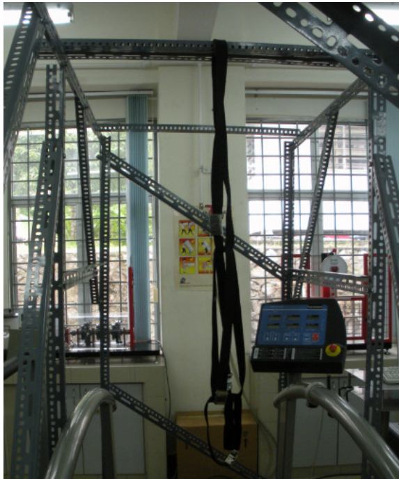
Figure 3.11: The safety belt is attached to the supporting structure
