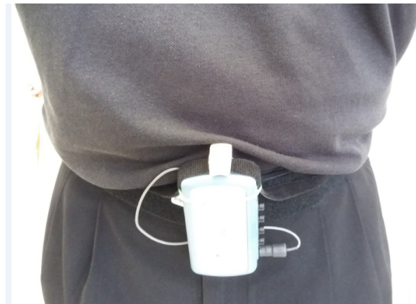
Figure 3.7: Subject wears the three axes wireless accelerometer at the waist position
