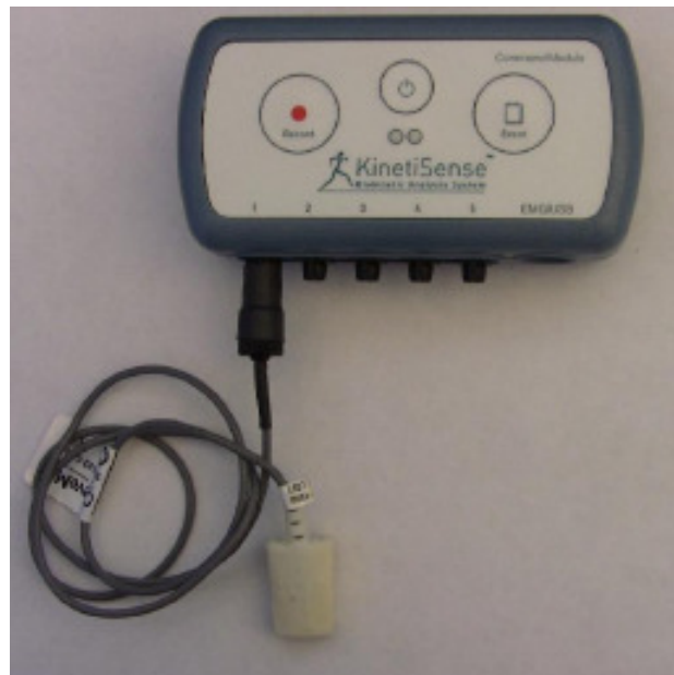
Figure 3.4: Tri-axial accelerometer is connected to command module using DIN connector
