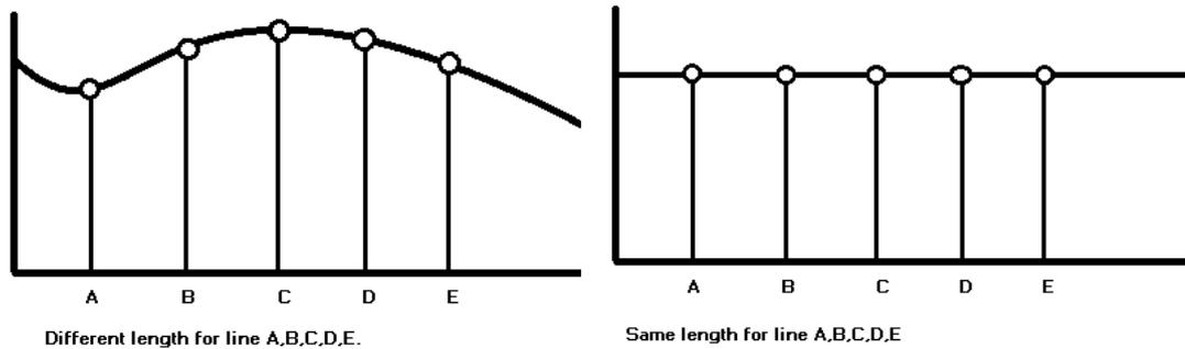
Figure 6.2 Curve Detection
