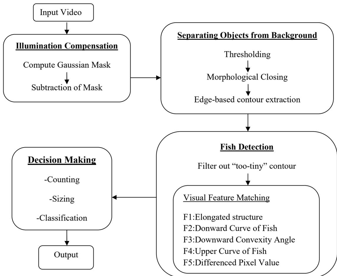
Figure 3.1 System Overview of Fish Monitoring System
