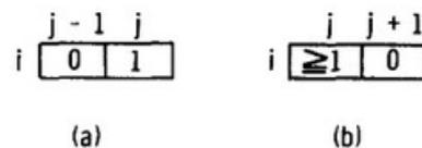
Figure 2.6 Conditions of border following, (a) for an outer border, (b) for a hole border
