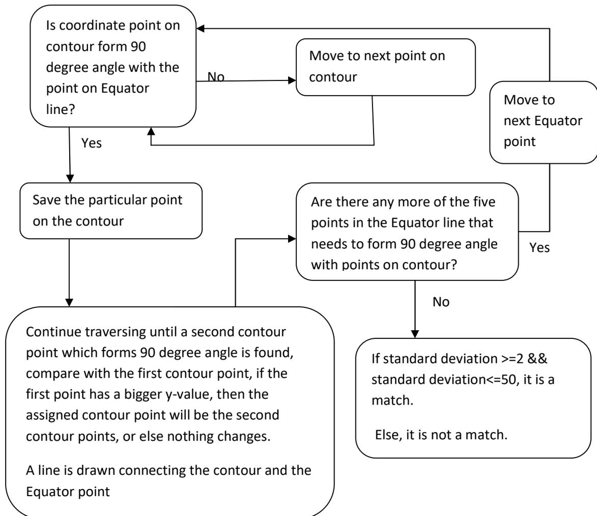
Figure 6.3 Overview of Curve Detection algorithm
