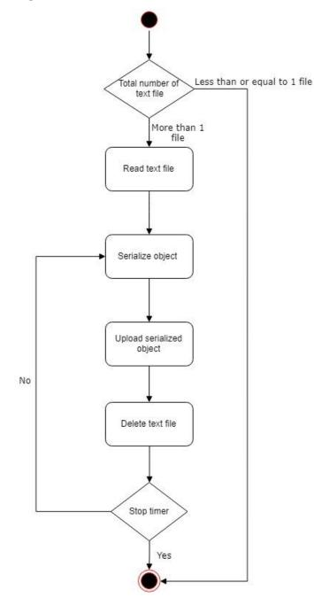
Figure 3.6 Data Upload Flowchart
