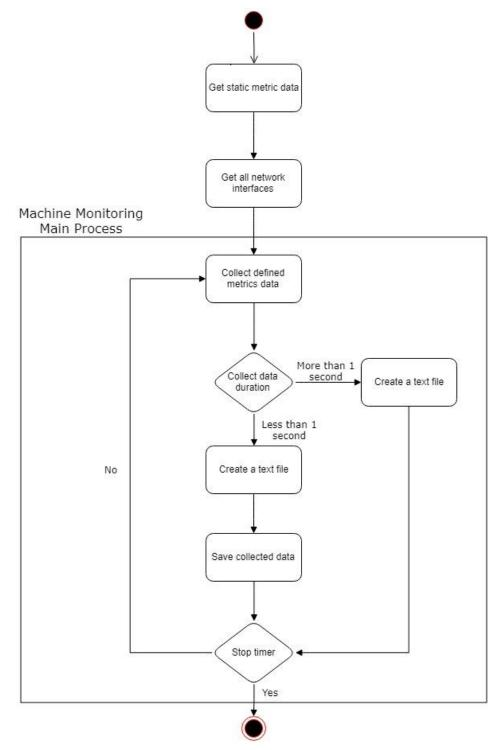
Figure 3.3 Machine Monitoring Thread
