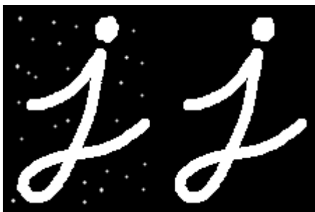
Figure 1.2-F7 Reducing noise using Opening (OpenCV dev team, 2014)
