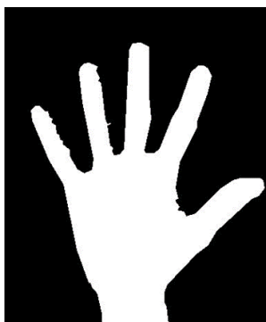
Figure 1.2-F5 Hand Region after Thresholding (Definition, 2013)
