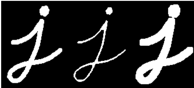
Figure 1.2-F6 Threshold image after perform Erosion and Dilation (OpenCV dev team, 2014)
