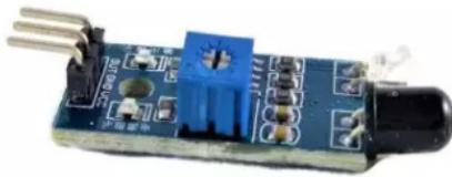
**IR Infrared Obstacle Avoidance Sensor**
