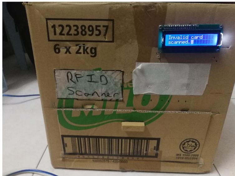
**Figure 6.17 Invalid Card Scanned**
