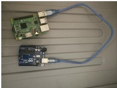
**Figure 6.3 Serial Port Communication of Raspberry Pi with Arduino Board**
