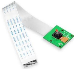
Figure 4.2.1.2.1 Raspberry pi camera module V1.3 with CSI ribbon cable
