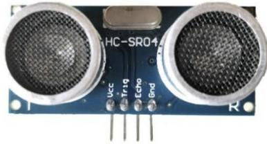
Figure 4.2.1.6.1 HC-SR04 Ultrasonic sensor
