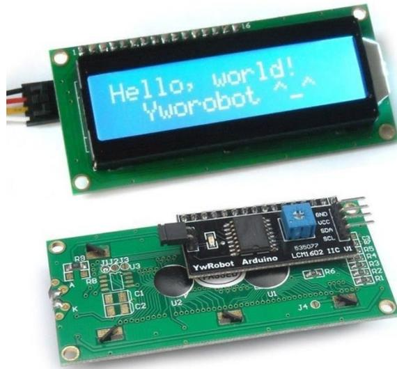
Figure 4.2.1.3.1 LCD1602 display with I2C LCD controller
