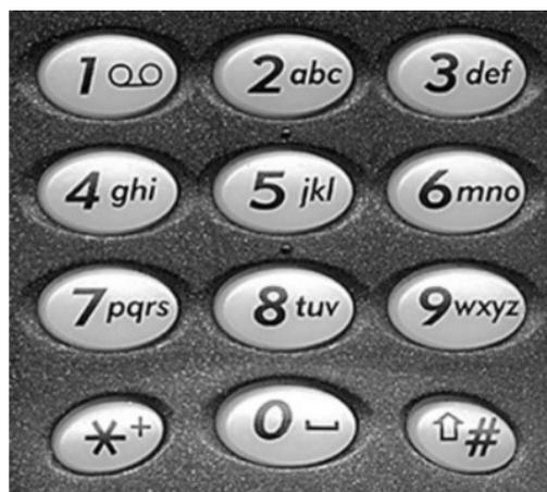
**Figure 1-3:** The 12-Key keypad on a mobile device
