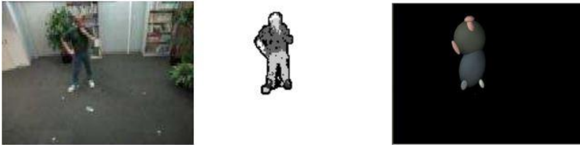
Figure 2.1: (left) video input (color image), center: segmentation, right: a 2-D blob statistic model represents human body
