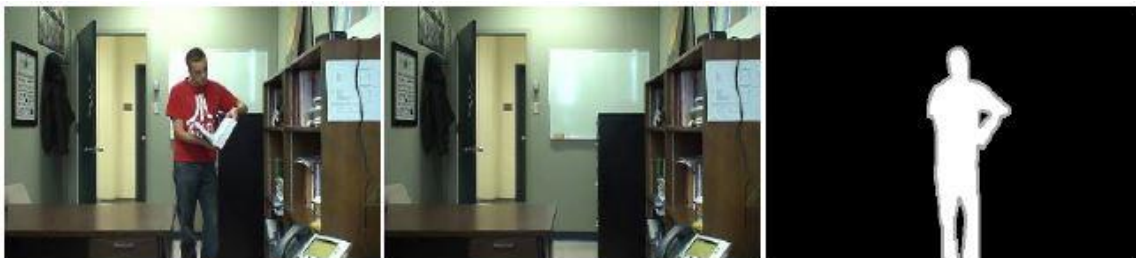
Figure 2.0: Background subtraction example for two sequence frame in an ‘office’. Left: frame number, Middle: background scene, Right: ground truth foreground mask
