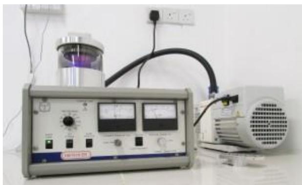
Figure 3.5: Sputter Coater (Model: SC7620, Emitech)
