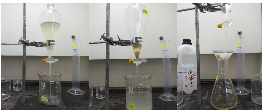
Figure 3.10: Oil Extraction Process (a) Experimental Setup, (b) Separation of Water Layer and Solvent Layer, (c) Drip-draining of Solvent Through Glass Funnel
