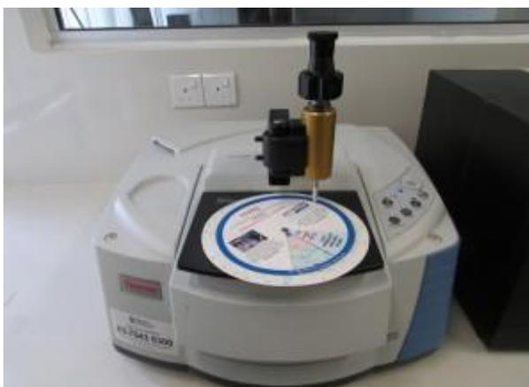
Figure 3.7: Fourier Transform Infrared Spectrometer (Model: Nicolet iS10, Thermo Scientific)
