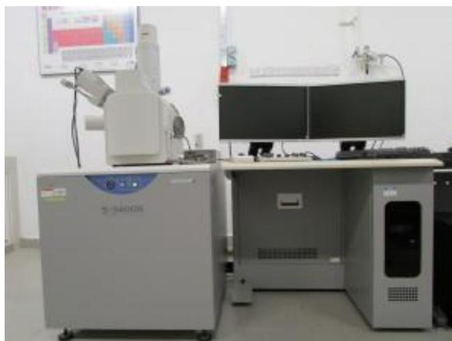
Figure 3.6: Scanning Electron Microscope (Model: S-3400, Hitachi)
