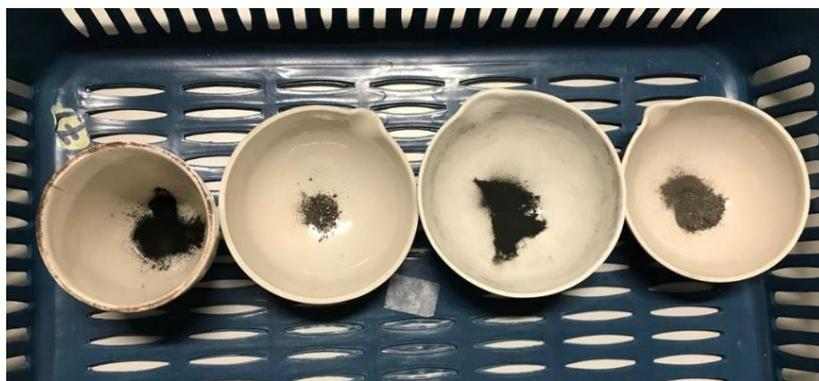
**Figure 3.2: Dried acetone-washed spent catalysts collected from hydrogenated citral, CPO, lauric acid and SPSFA (from left to right).**
