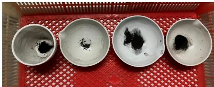
**Figure 3.3: Roasted acetone-washed spent catalysts collected from hydrogenated citral, CPO, lauric acid and SPSFA (from left to right).**
