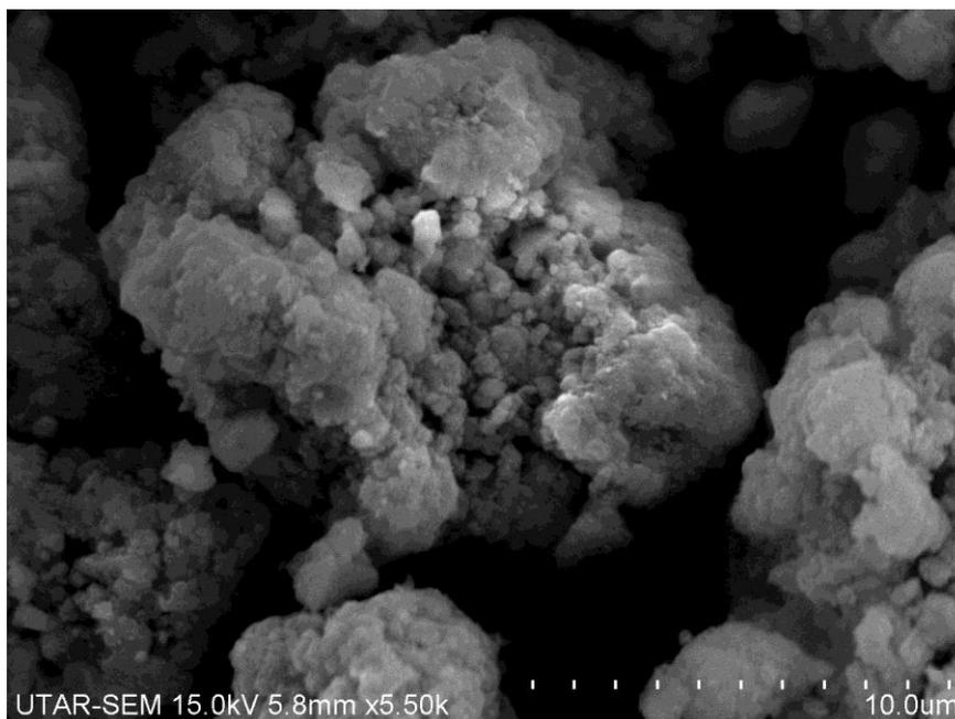
**Figure 4.1: SEM image of fresh Ni/SiO<sub>2</sub> catalyst (magnification x5500)**
