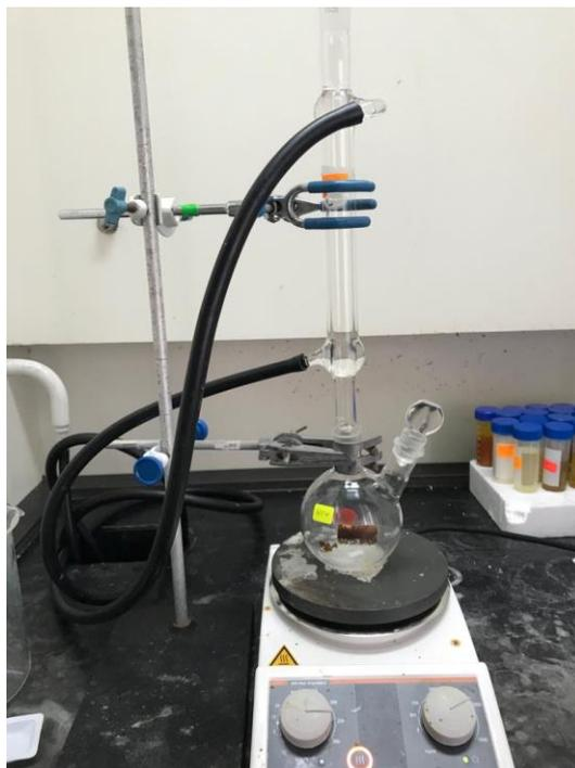
**Figure 3.4: Esterification of fats under reflux**
