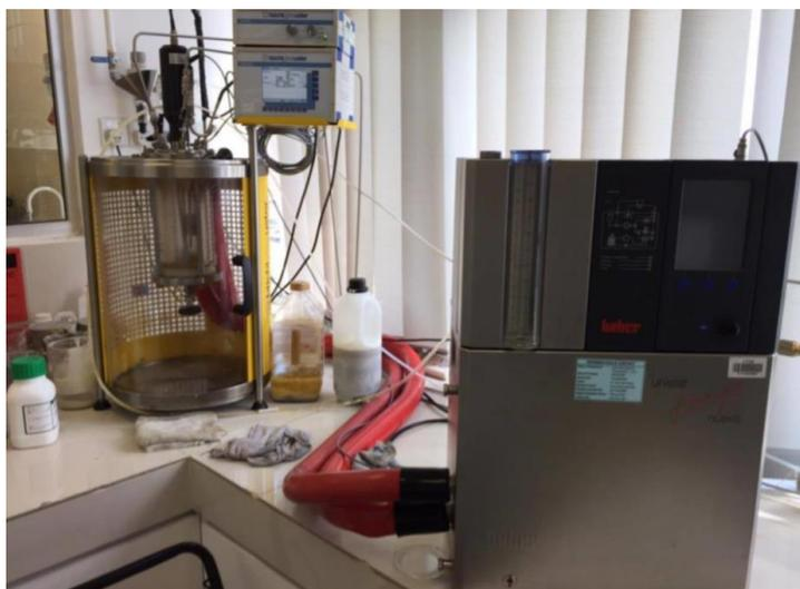
**Figure 3.1: Reactor for Hydrogenation Process**
