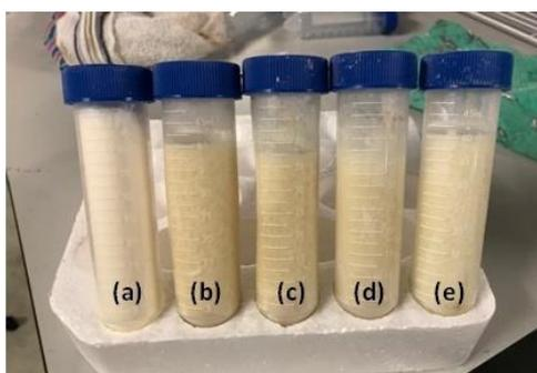
**Figure 4.8: Lauric acid before (a) and after 30 minutes, 60 minutes, 120 minutes and 180 minutes (b, c, d, e) hydrogenation reaction, respectively.**
