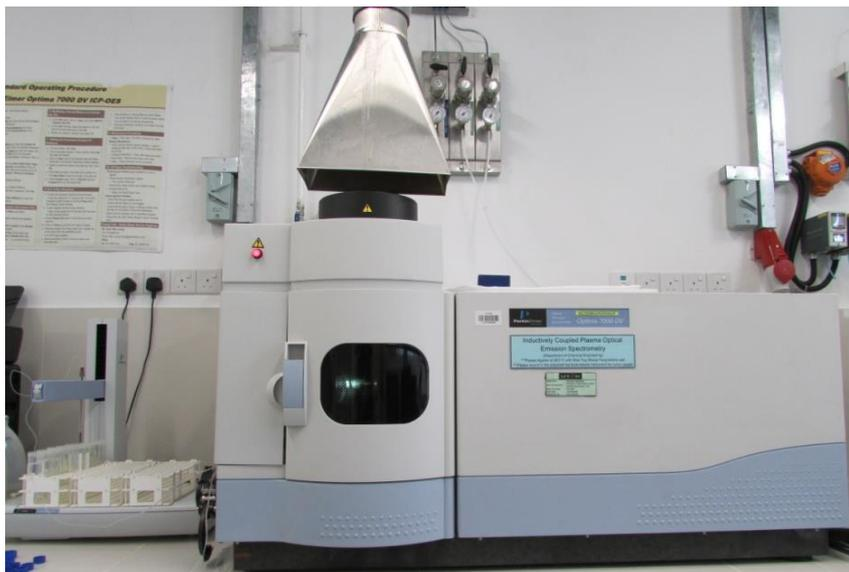
**Figure 3.11: PerkinElmer optical emission spectrometer Optima 7000 DV**
