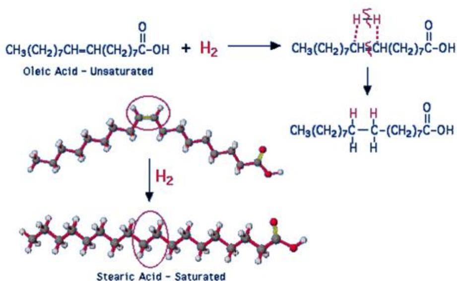
**Figure 2.13: Hydrogenation of Oleic Acid (Ophardt, 2003)**
