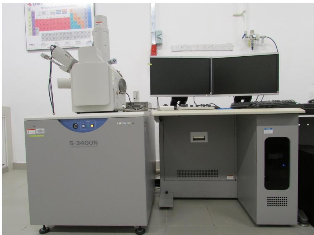
**Figure 3.10: Hitachi S-3400N scanning electron microscope**
