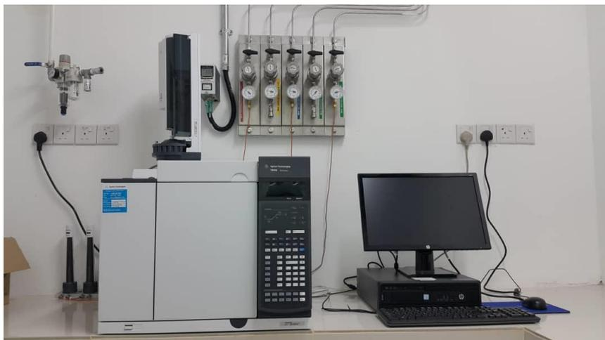
**Figure 3.9: Agilent Technologies 7890B Gas Chromatography**
