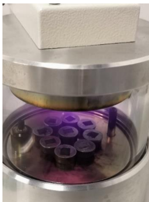
Figure 3.5: Coating of Electric-conducting Material (Gold Film)
