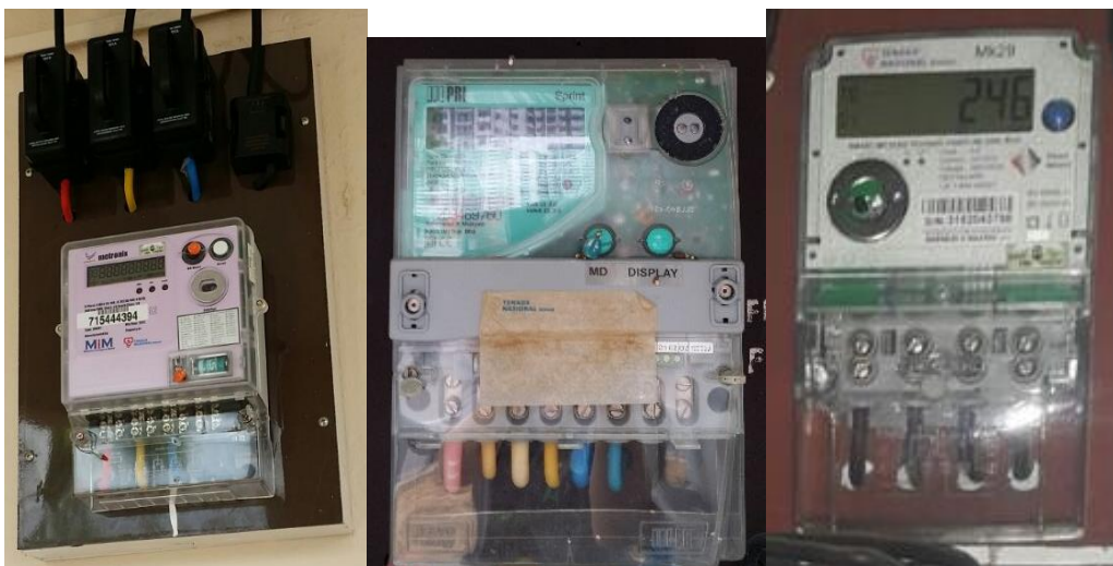
Group of the three brands of smart meters which are from left to right ; - Metronix, Sprint, and Mk29.
