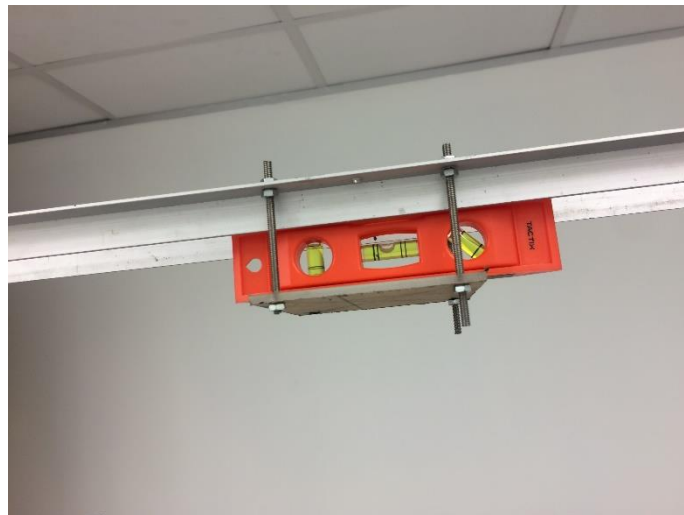
Figure 3.7: Levelling of Target Board Using Spirit Leveller
