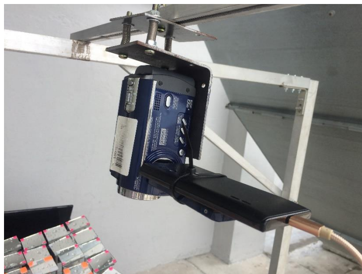
Figure 3.9: Levelling of Camera Lens Using Smartphone Levelling Function
