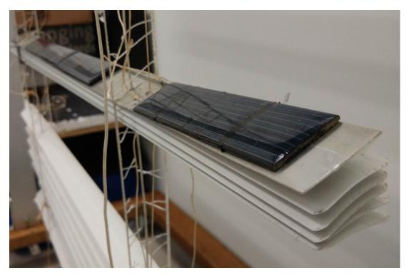
Figure 4.3 Gap to Minimize Mutual Shading
