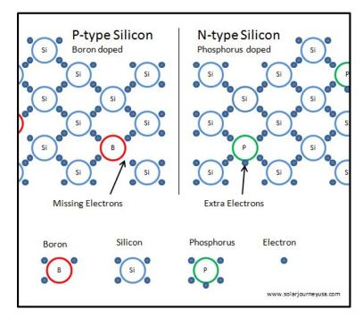
Figure 2.8 Crystalline Structure of Silicon
