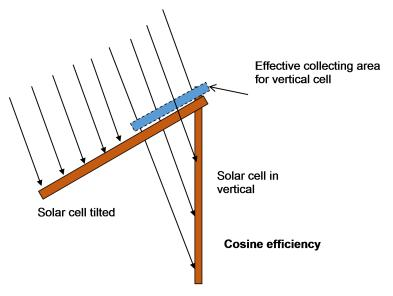
**Figure 1.4 Illustration of Cosine Effect**
