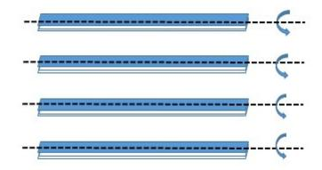
Figure 3.3 Gaps to Avoid Mutual Shading
