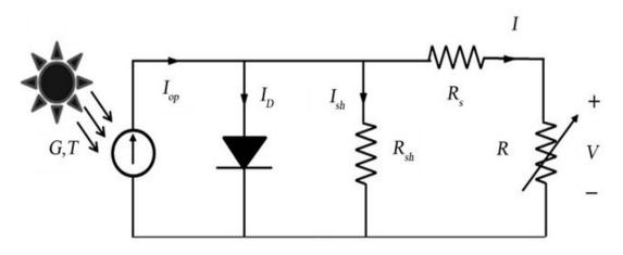
Figure 2.11 Solar Cell Equivalent Circuit (Nur Mohammad, 2013)
