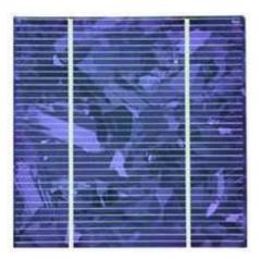
Figure 2.3 Polycrystalline Silicon Cell
