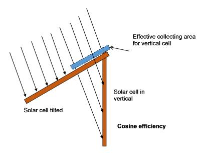
**Figure 2.15 Cosine Efficiency**
