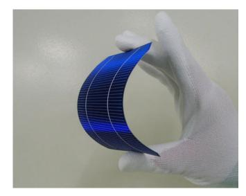
Figure 2.4 Thin-film Cell Technology
