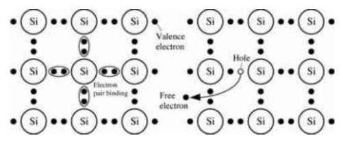
Figure 2.7 Crystal Structure of Silicon and Intrinsic Conductivity
