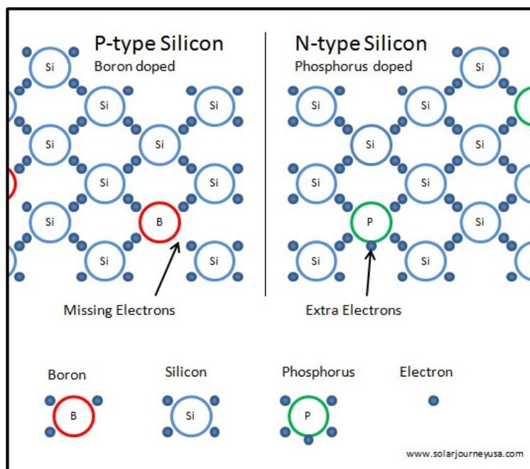
**Figure 2.8 Crystalline Structure of Silicon**
