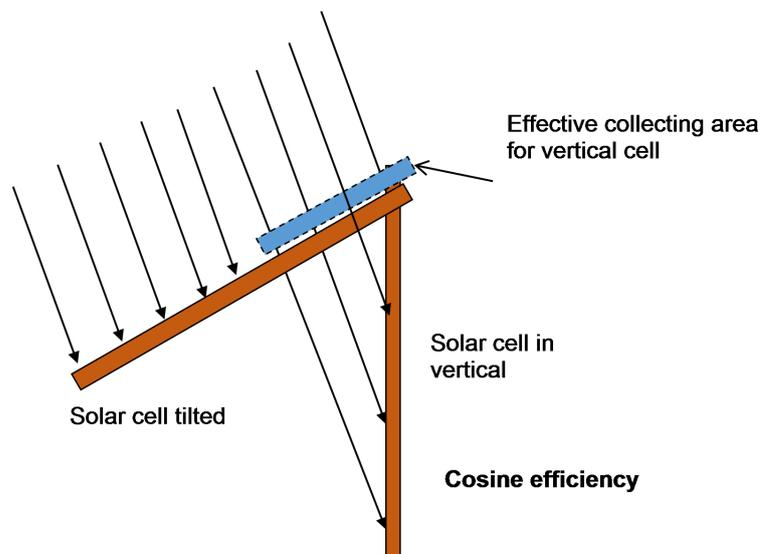
**Figure 1.4 Illustration of Cosine Effect**
