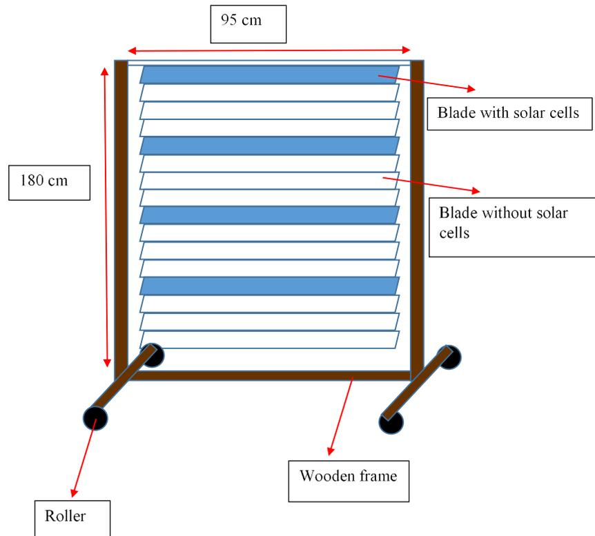
**Figure 3.2 Prototype Design**
