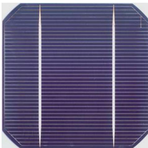
**Figure 2.1 Semi-square Monocrystalline Cell**
