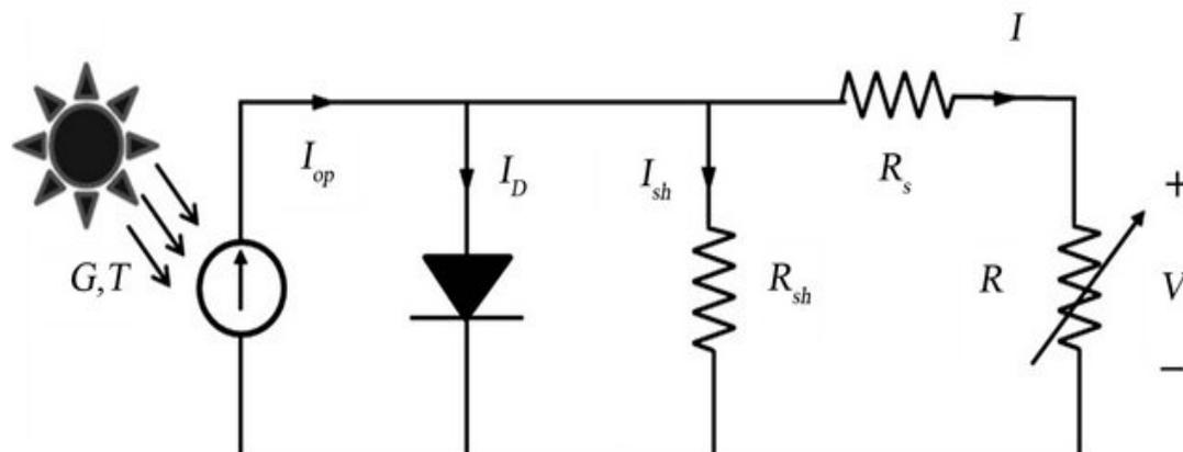
Figure 2.11 Solar Cell Equivalent Circuit (Nur Mohammad, 2013)
