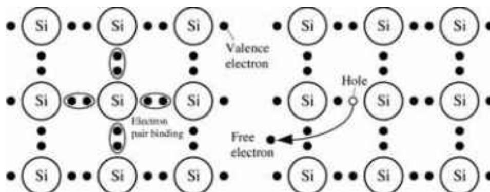
**Figure 2.7 Crystal Structure of Silicon and Intrinsic Conductivity**
