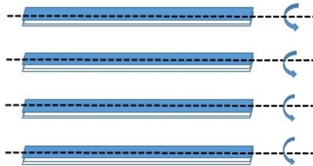
**Figure 3.3 Gaps to Avoid Mutual Shading**
