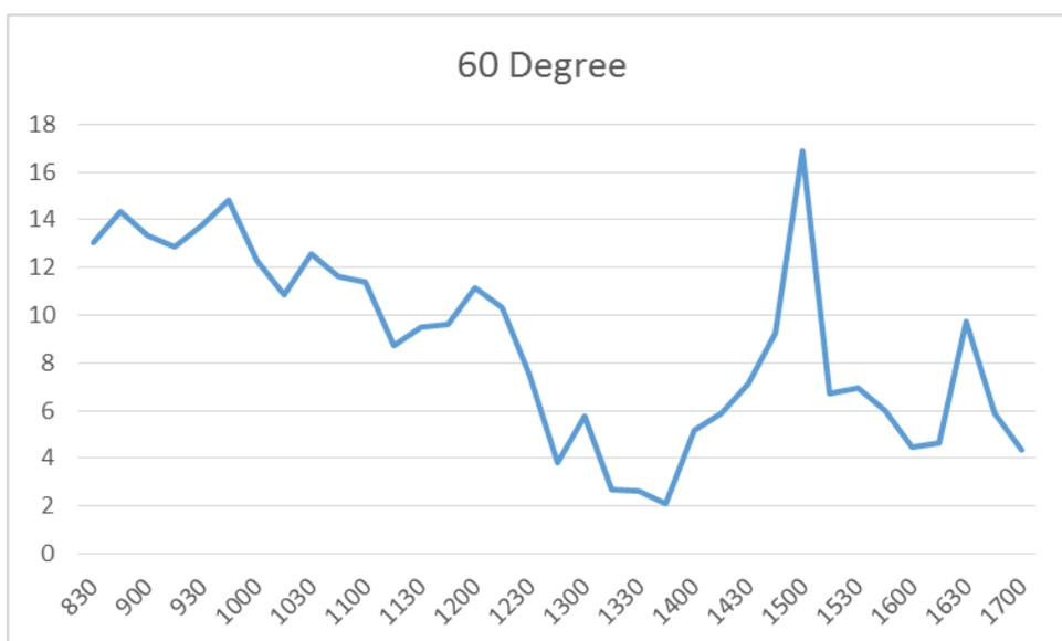
**Figure 4.9 Power per 1000W/m² vs Time (3-8-2016)**
