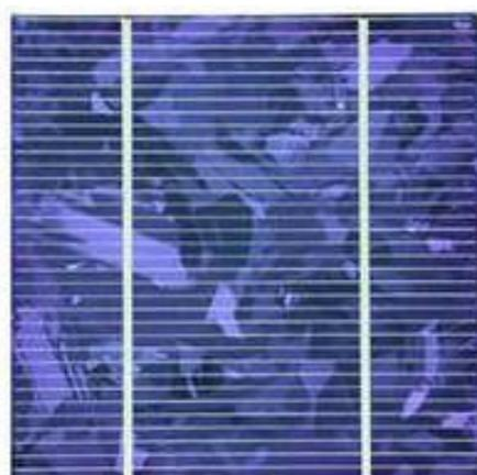
**Figure 2.3 Polycrystalline Silicon Cell**
