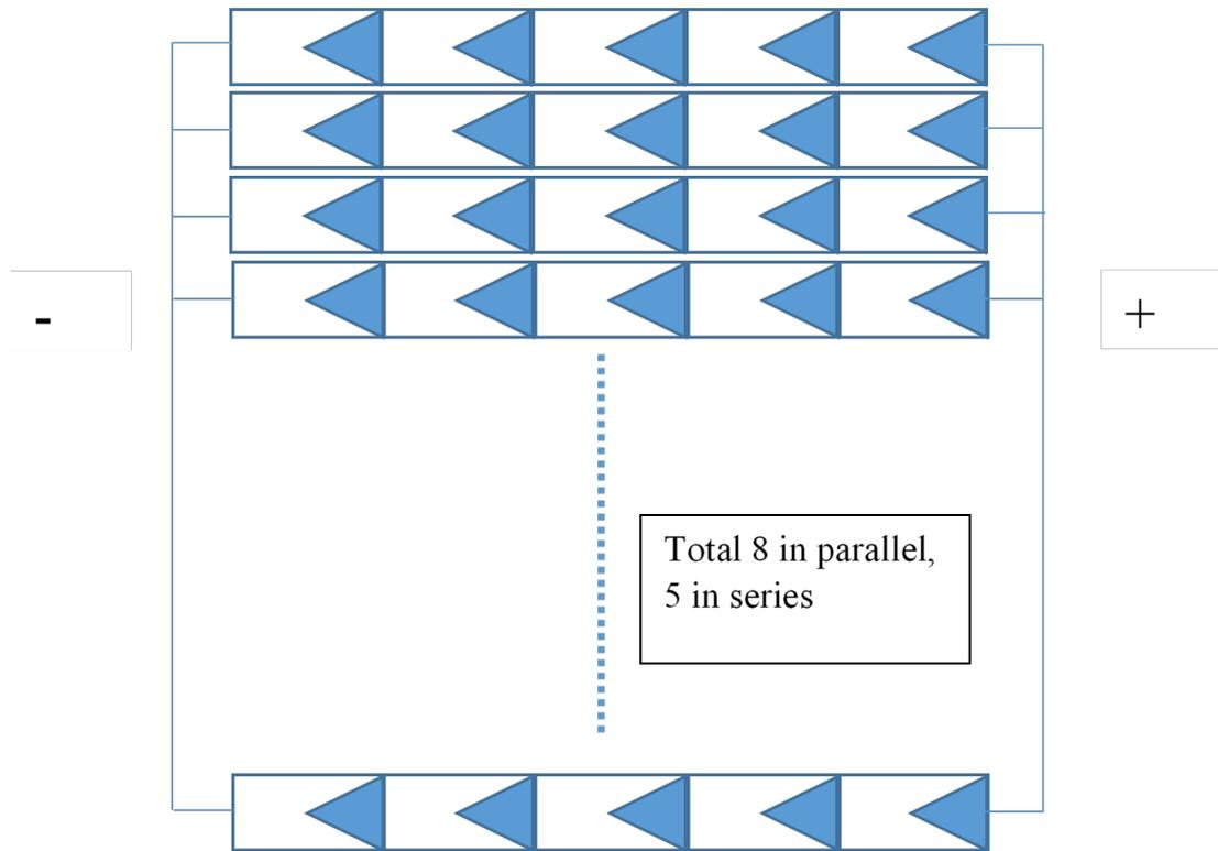
**Figure 3.7 Circuitry Detail**
