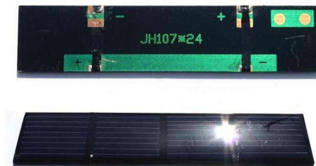
**Figure 3.1 C-Si Solar Cell**
