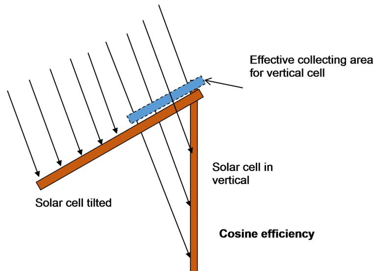
**Figure 2.15 Cosine Efficiency**
