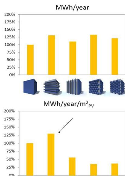
**Figure 2.16 Comparison between 5 Types of Facade (Sara Freitas, 2015)**
