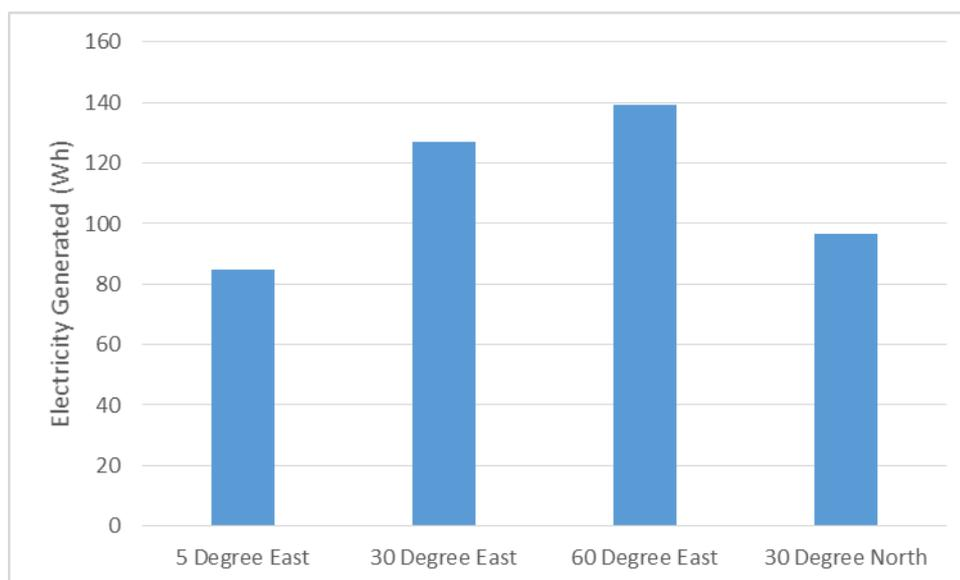
**Figure 4.17 Electricity Generated in Different Tilting Angles and Directions**
