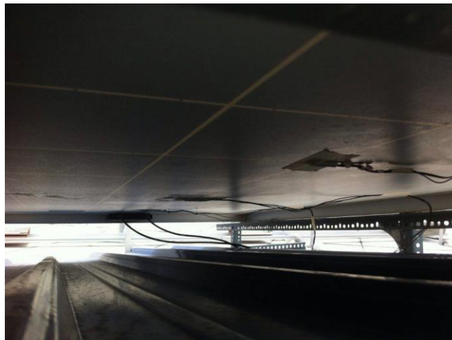
Figure 3.11: 3 DS18B20 Position Top, Middle and Bottom of the Solar Panel
