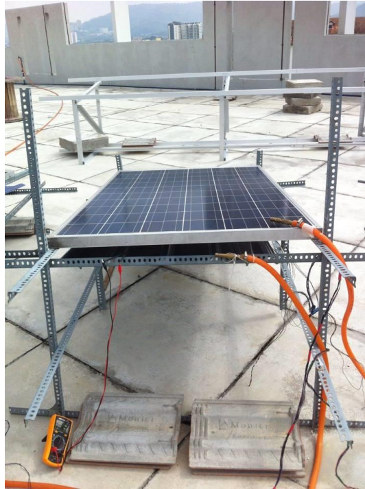
Figure 3.7: Water Hose Attached onto the Solar Panel
