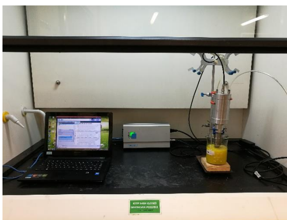
Figure 3.1: Set-up of Ultrasound Equipment
