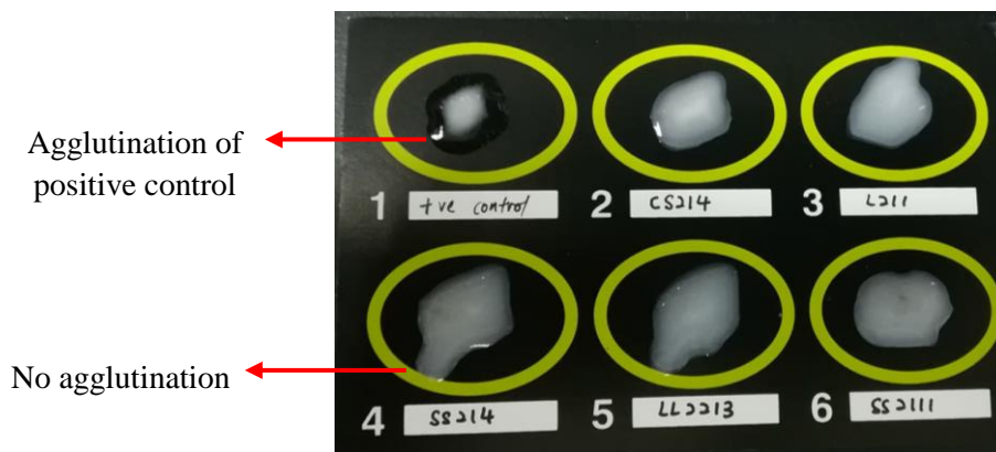
Figure 4.9: Result using ELISA Listeria Latex Kit. Well 1 sample is a positive control provided in the kit. Well 2 to 6 are bacterial isolates from this study.
