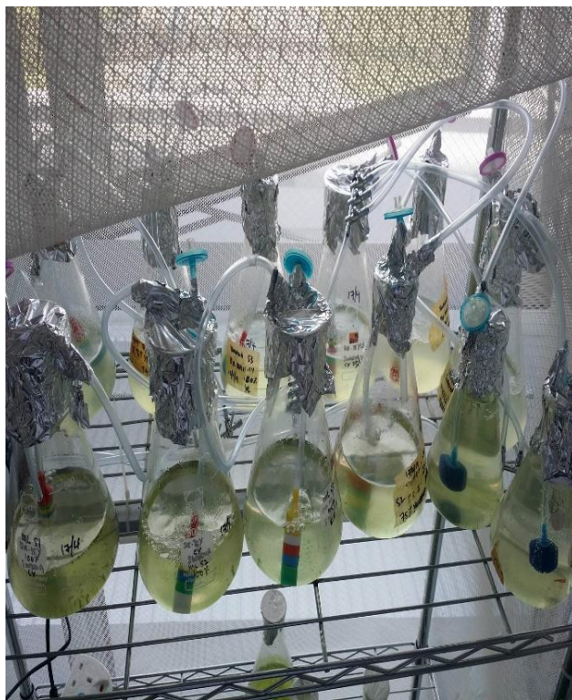
Figure 3.7 Chlorella vulgaris in mature leachate samples with aeration set-up.
