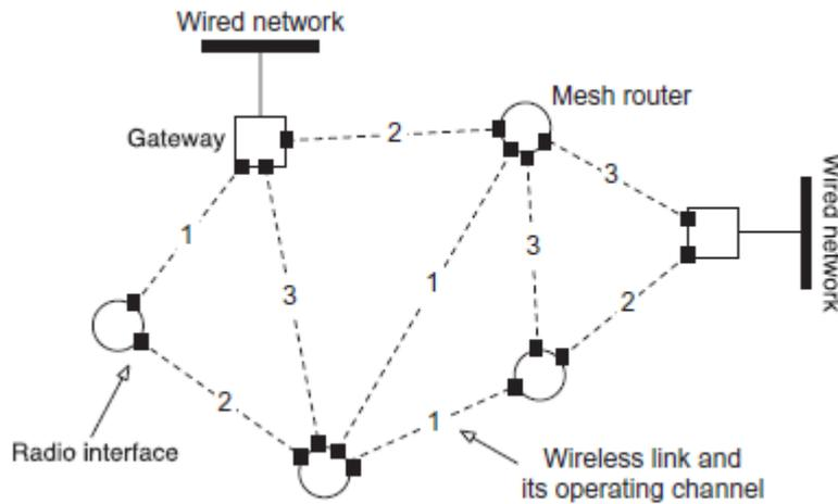
Figure A.1 A multi-radio wireless mesh network with channel assignment.
