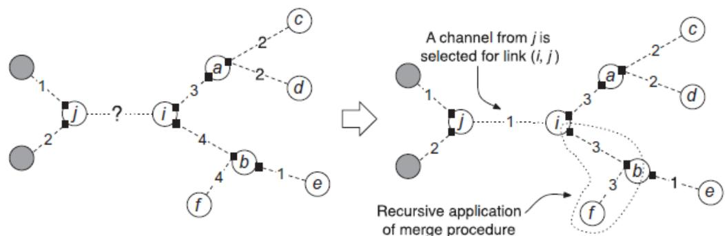
Figure A.5 Sample topology before and after a merge operation.
