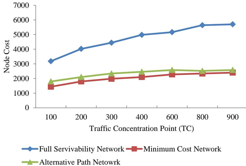
Figure 5.6: Node Cost normalized to that of an ONU for 500 Potential WR Installation Sites.
