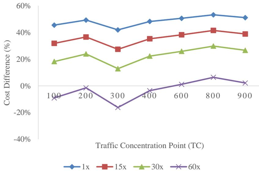
Figure 5.11: Cost Difference between FSN and APN for 400 Potential WR Installation Sites.
