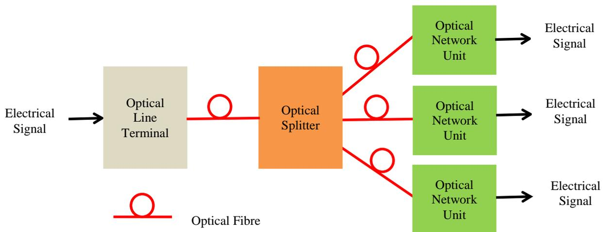
Figure 2.2: Network architecture of a Passive Optical Network (PON).
