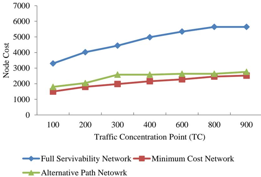
Figure 5.5: Node Cost normalized to that of an ONU for 400 Potential WR Installation Sites.
