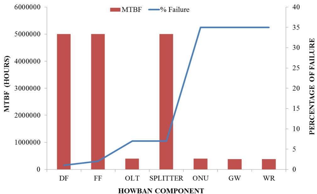
FIGURE 4.2: Comparison of MTBF and Failure Statistics of network component.
