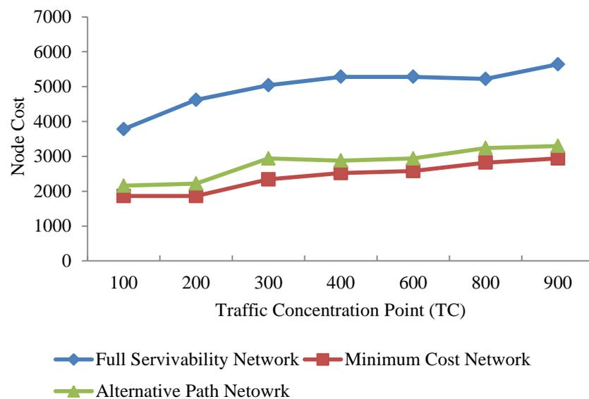
Figure 5.3: Node Cost normalized to that of an ONU for 200 Potential WR Installation Sites.
