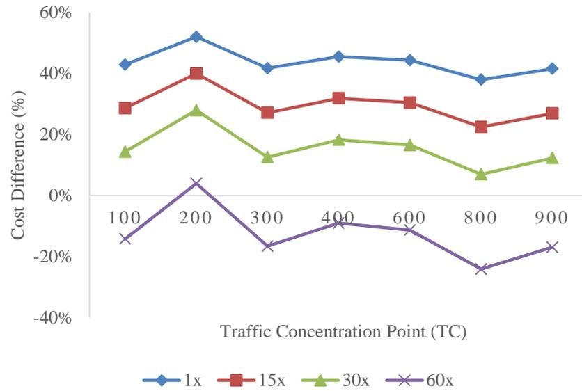
Figure 5.9: Cost Difference between FSN and APN for 200 Potential WR Installation Sites.
