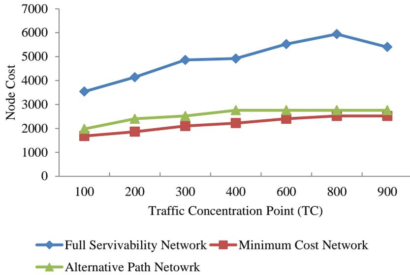
Figure 5.4: Node Cost normalized to that of an ONU for 300 Potential WR Installation Sites.
