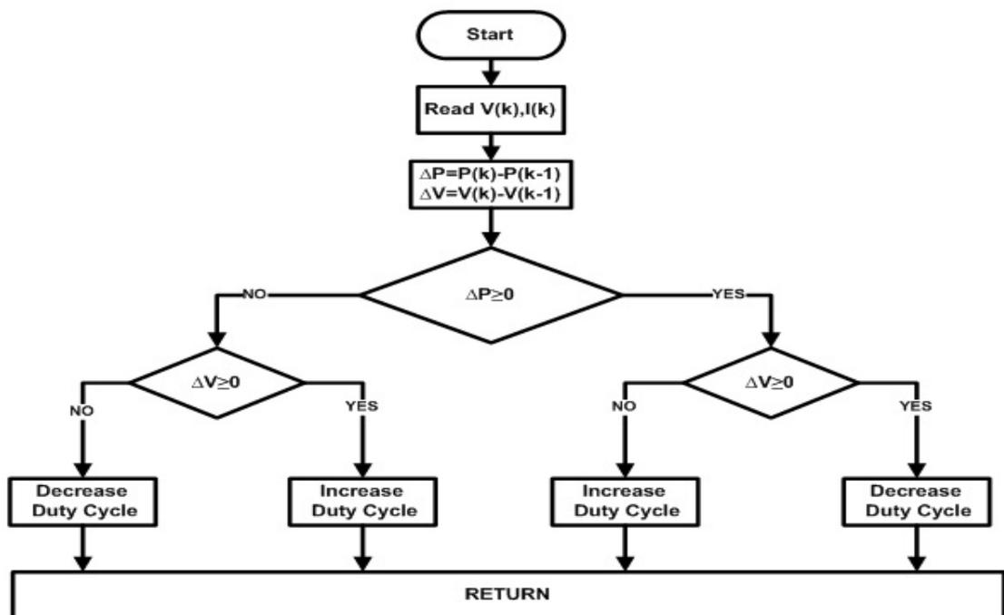
Figure 2-11 P&O algorithm flowchart
