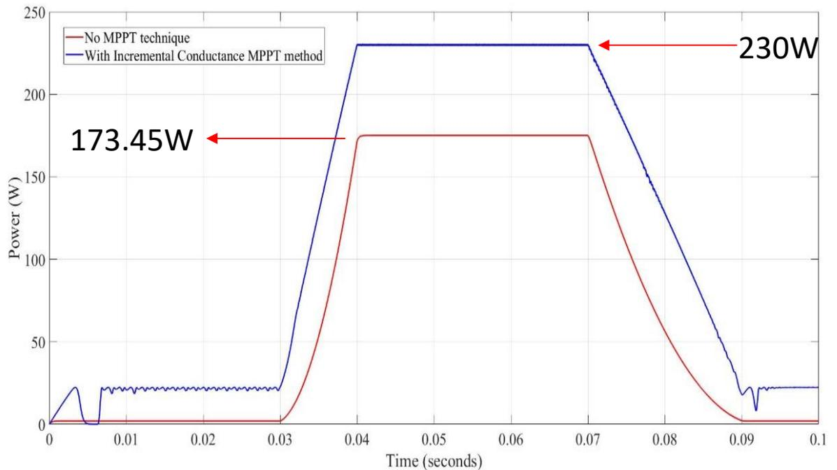
Figure 4-2 PV module power with Incremental Conductance MPPT and without MPPT
