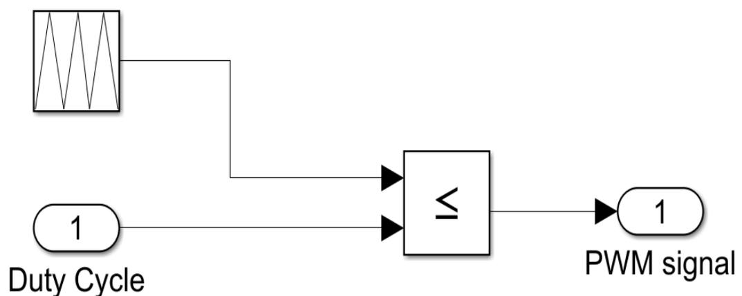
Figure 3-6 Comparator block to generate PWM signal for DC-DC Buck Converter
