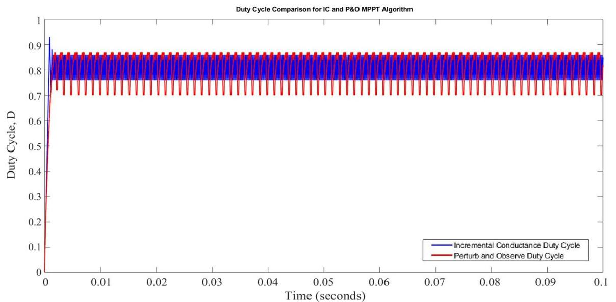
Figure 4-11 Duty cycle comparison between incremental conductance and perturb and observe
