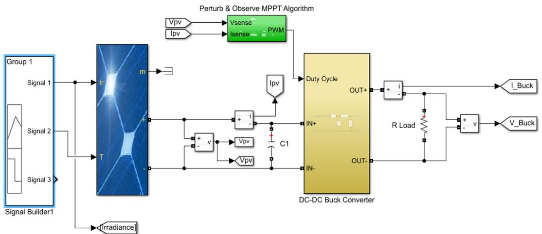
Figure 3-4 Perturb & Observe MPPT Algorithm with Buck Converter
