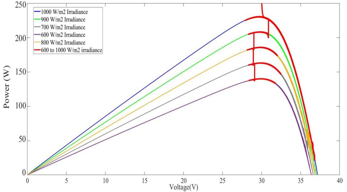
Figure 4-8 P&O Algorithm tracking from 1000 W/m<sup>2</sup> to 600 W/m<sup>2</sup>
