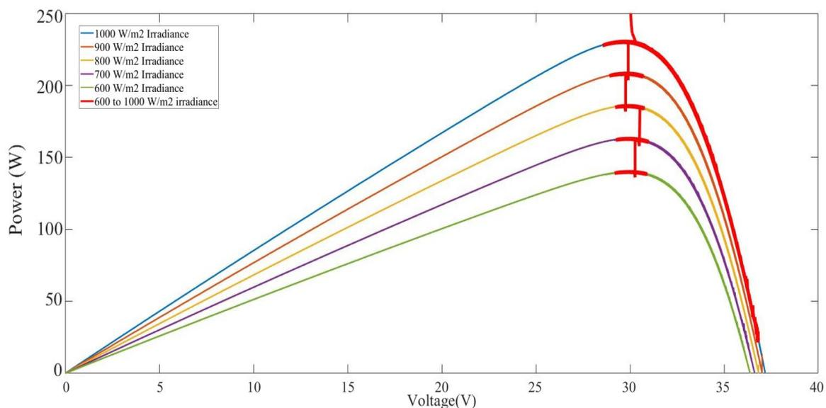
Figure 4-7 Incremental Conductance Algorithm tracking from  $1000\text{ W/m}^2$  to  $600\text{ W/m}^2$
