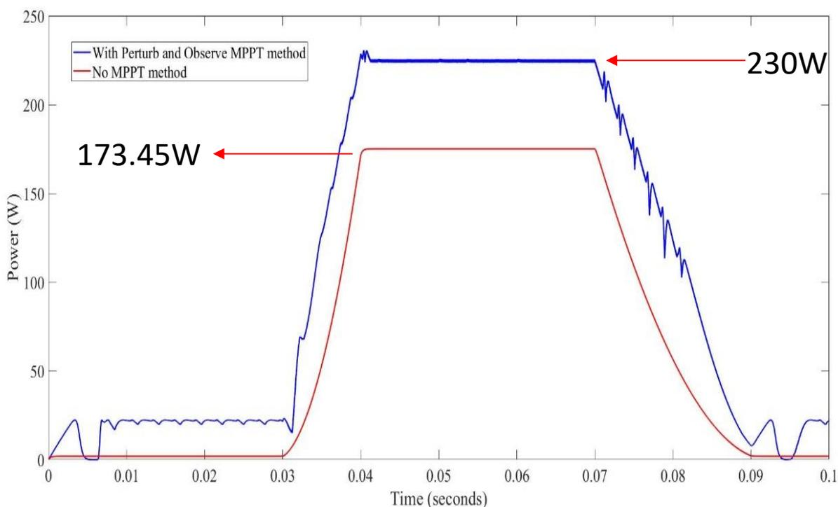
Figure 4-1 PV module power with P&O MPPT and without MPPT
