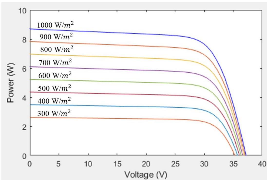
Figure 2-5 I-V Characteristic curve of PV model at varying irradiance at ambient temperature of  $25^\circ\text{C}$
