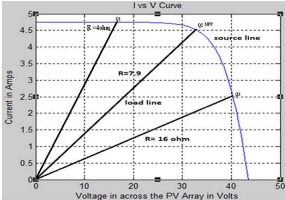
Figure 2-16 IV Curve and load line for solar module at various loads. (Pradhan and Panda, 2005)
