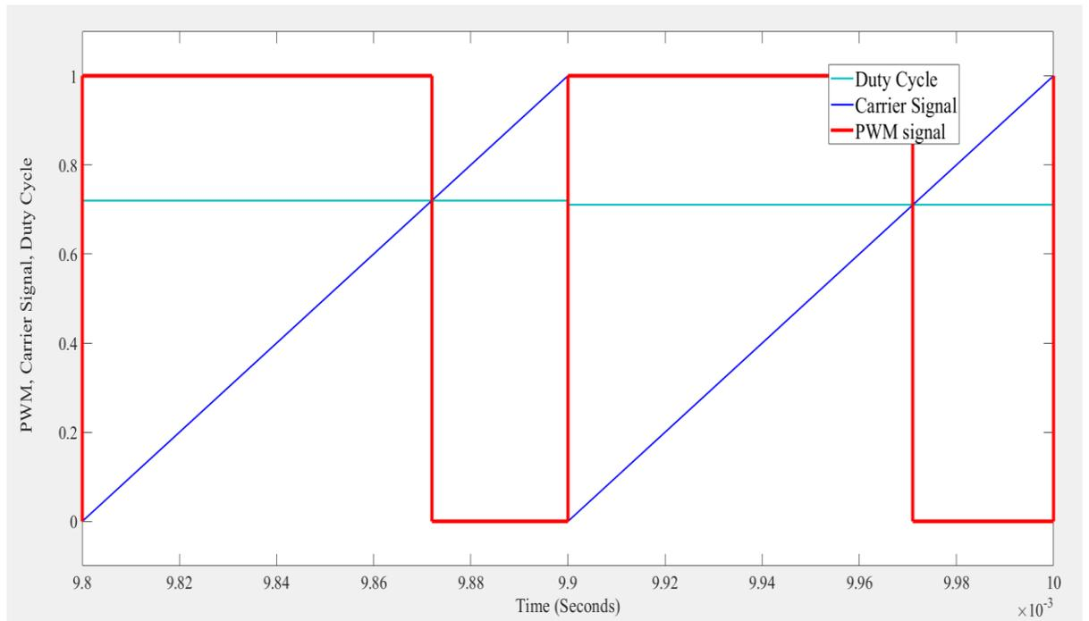
Figure 3-7 PWM Signal Generated from comparison of Triangle Signal and Duty Cycle
