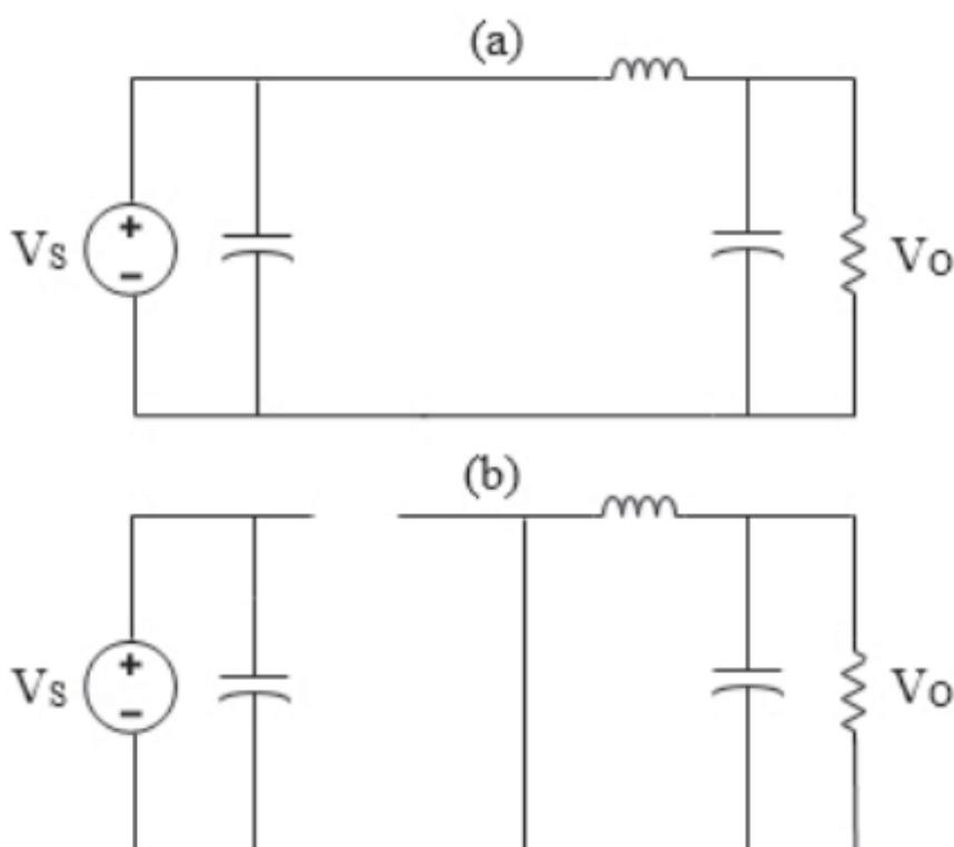
Figure 2-15 (a) Buck Converter during switch turned ON and (b) Buck Converter during switch turned OFF
