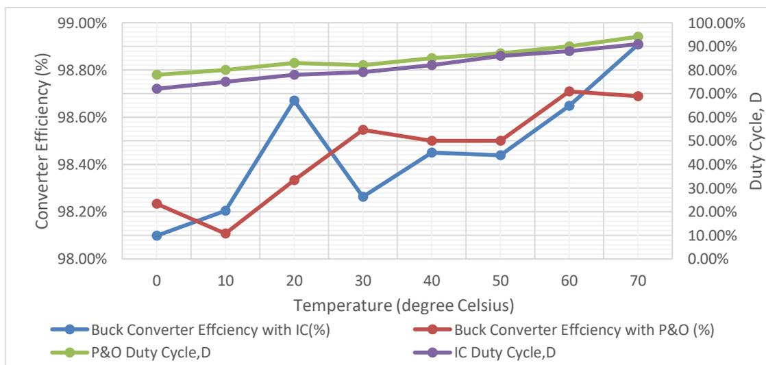
Figure 4-10 Comparison of buck converter efficiency and duty cycle of Incremental Conductance and Perturb and Observe MPPT algorithm with varying temperature and fixed  $1000 \text{ W/m}^2$  irradiance.
