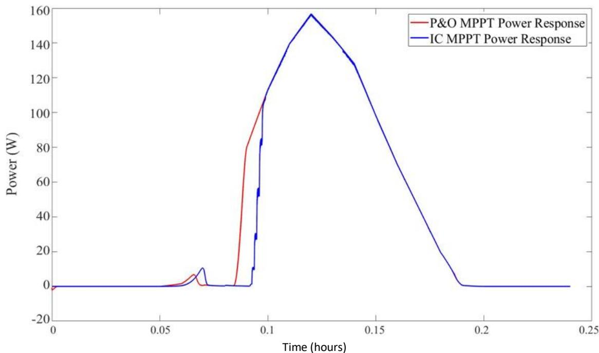
Figure 4-6 Power output curve for change in duty cycle perturbation step size for P&O and IC algorithm
