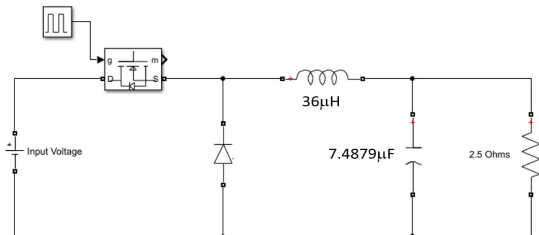
Figure 3-3 Buck Converter schematic to generate maximum load voltage of 24V
