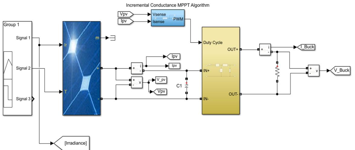
Figure 3-5 Incremental Conductance MPPT Algorithm with Buck Converter
