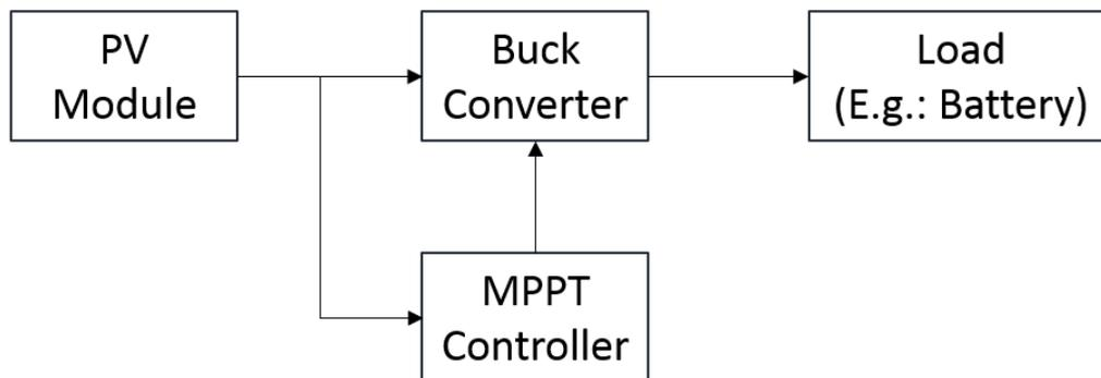
Figure 3-1 Block diagram of MPPT controller
