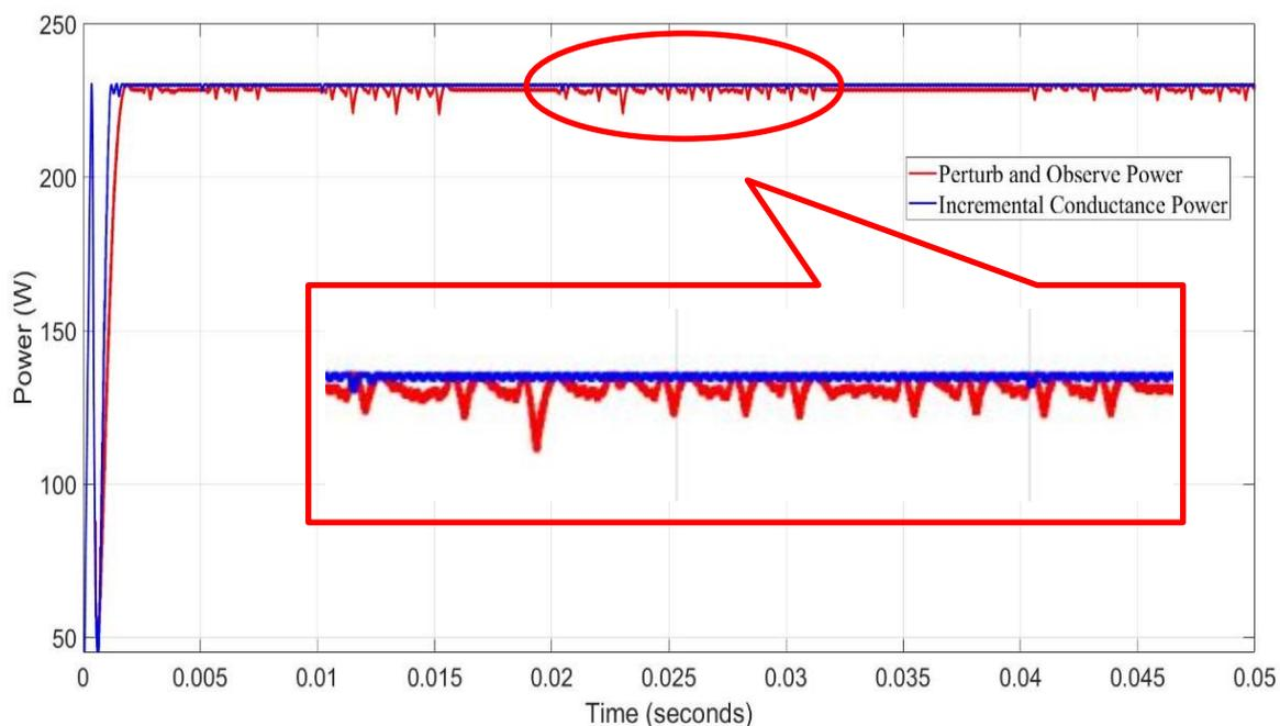
Figure 4-3 Power Output curve for Incremental Conductance and Perturb and Observe
