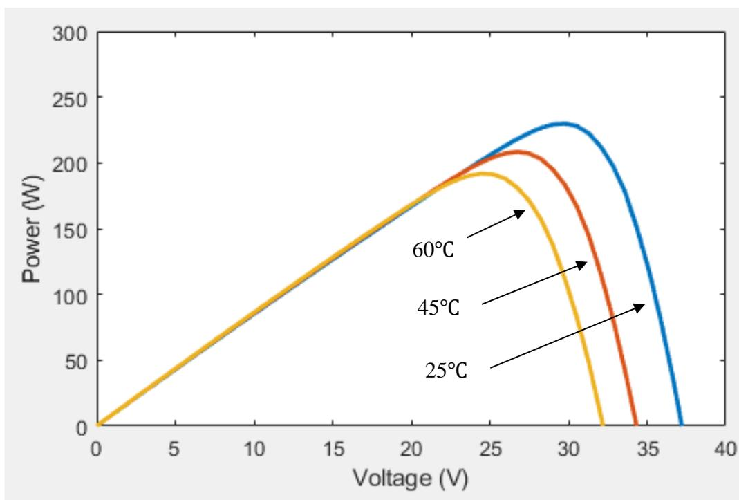
Figure 2-9 P-V Characteristics curve for PV model at varying temperature with fixed irradiance of 1000 W/m<sup>2</sup>
