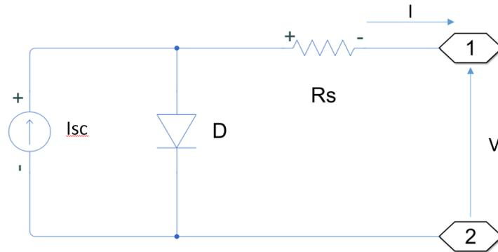
Figure 2-1 Single Diode Solar Cell Model
