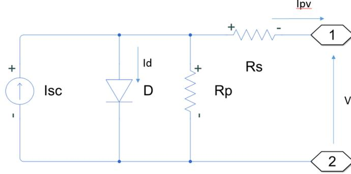
Figure 2-2 Solar cell model using single diode with  $R_s$  and  $R_p$
