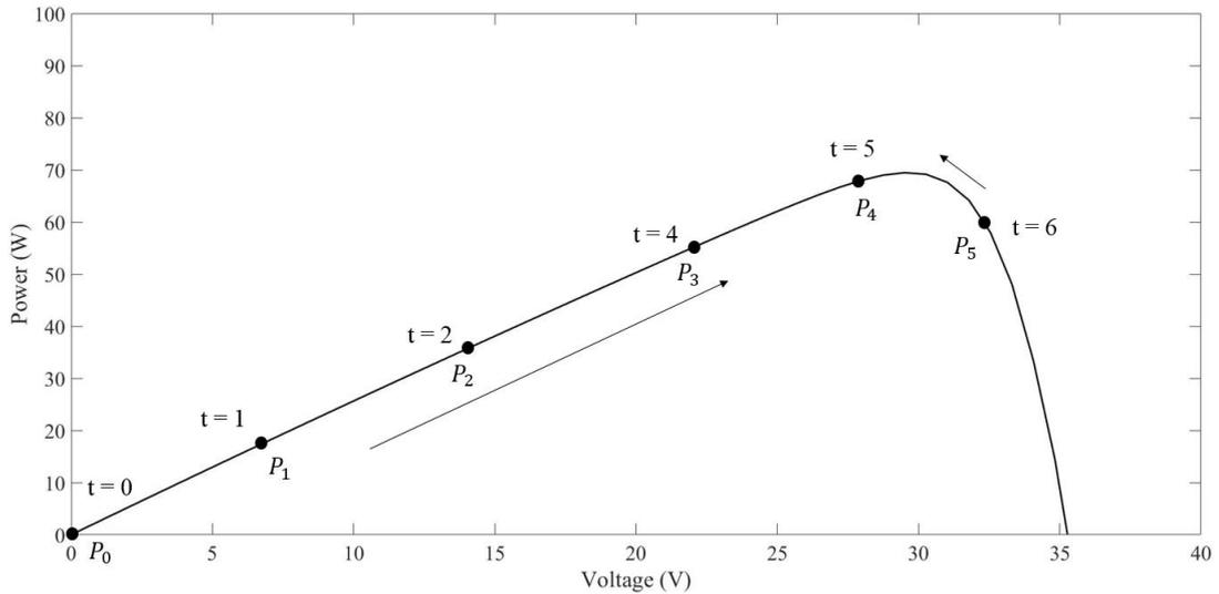
Figure 2-12 Perturb and Observe Tracking steps
