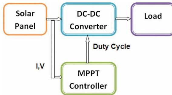
Figure 2-10 PV Panel system with MPPT and DC-DC Converter system block
