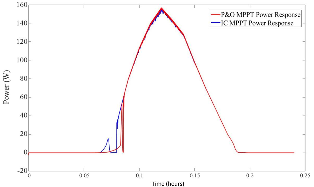
Figure 4-5 Real world irradiation and temperature testing for both MPPT algorithms
