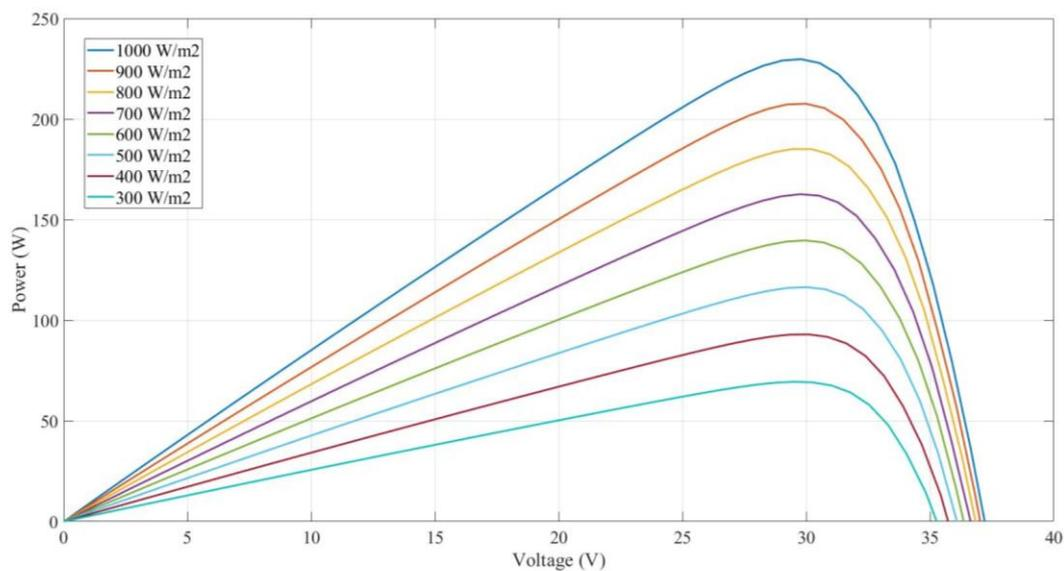
Figure 2-8 P-V Characteristics curve for PV model at varying irradiance and fixed 25°C
