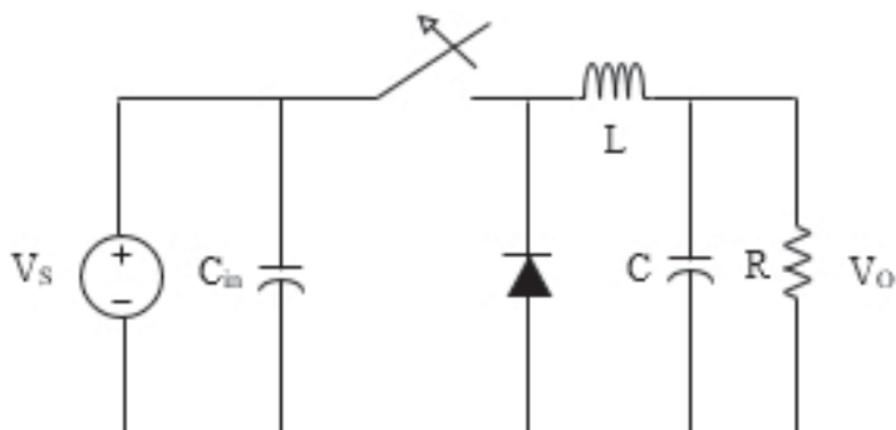
Figure 2-14 Buck Converter schematic
