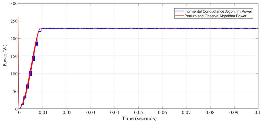
Figure 4-12 Power response comparison between incremental conductance and perturb and observe with smaller duty cycle perturbation step
