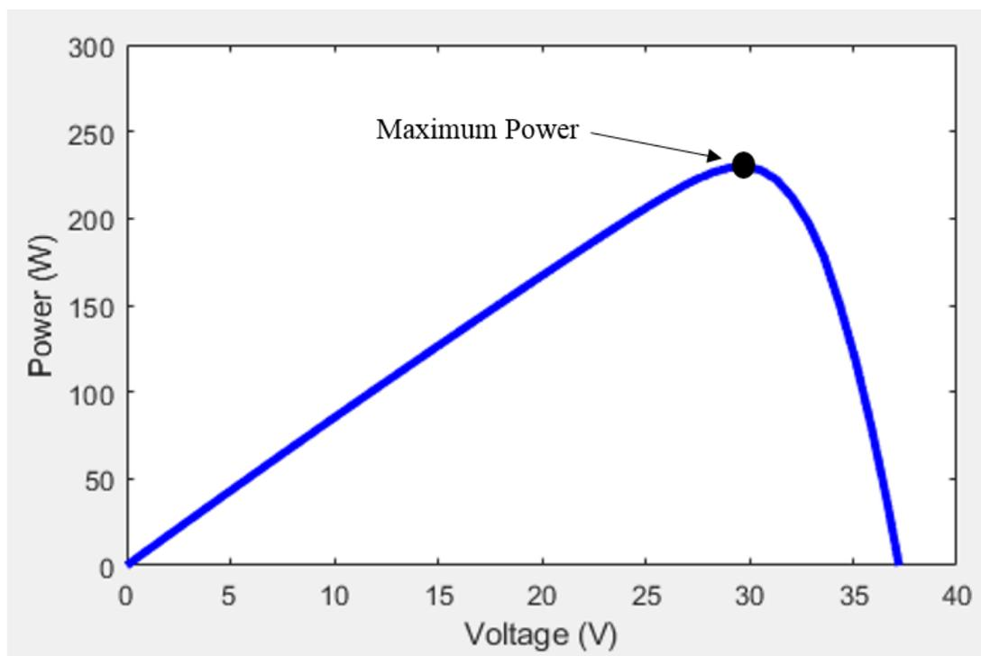
Figure 2-7 P-V Characteristic curve of PV model at  $1000 \text{ W/m}^2$  constant irradiance and ambient temperature of  $25^\circ\text{C}$
