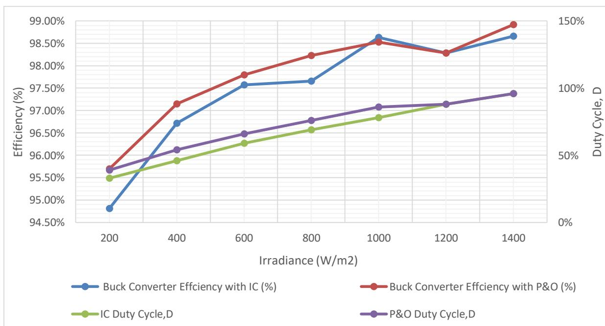
Figure 4-9 Comparison of buck converter efficiency of Incremental Conductance and Perturb and Observe MPPT algorithm with varying irradiance and fixed 25°C operating temperature
