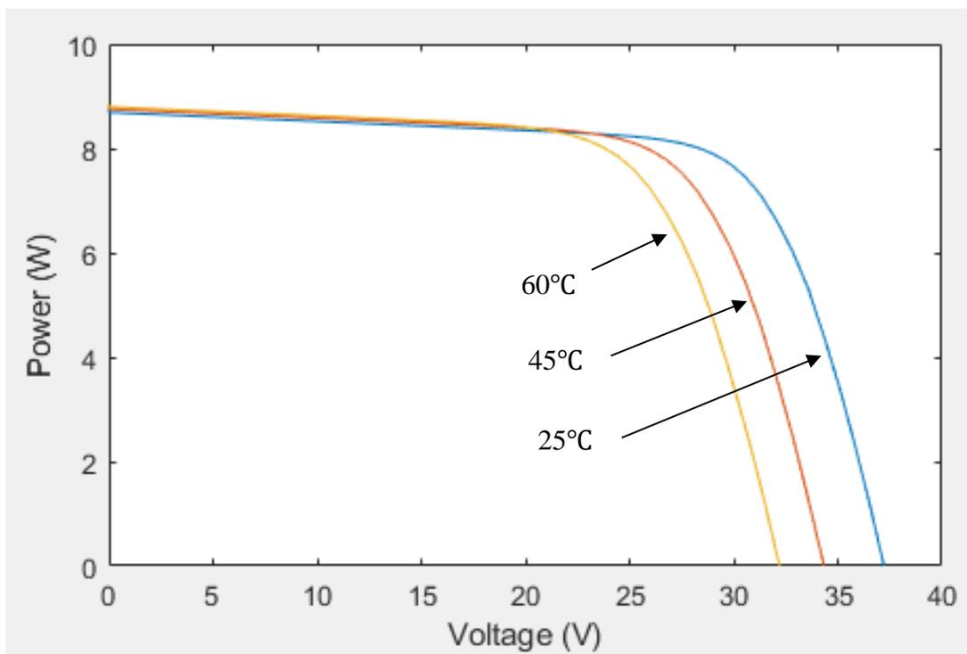
Figure 2-6 I-V Characteristic curve of PV model at varying temperature at constant irradiance of  $1000 \text{ W/m}^2$
