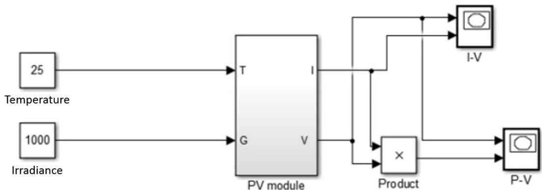
Figure 2-3 Simulink simulation schematic of PV model.
