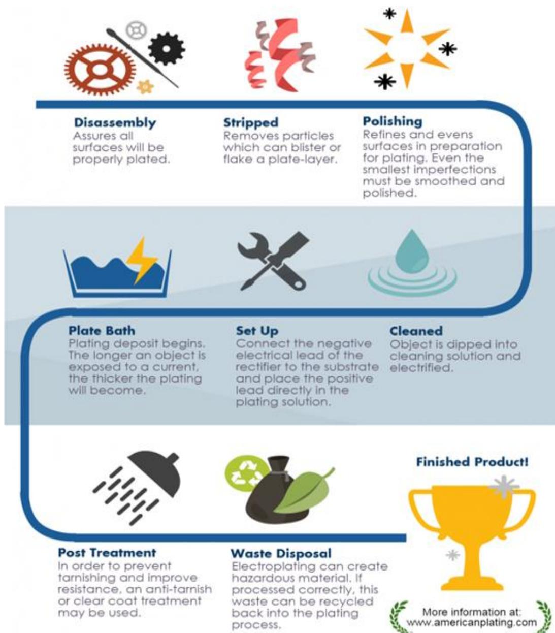
Figure 2.1: Simplified Diagram of Industrial Electroplating Process (American Plating Company, n.d.)
