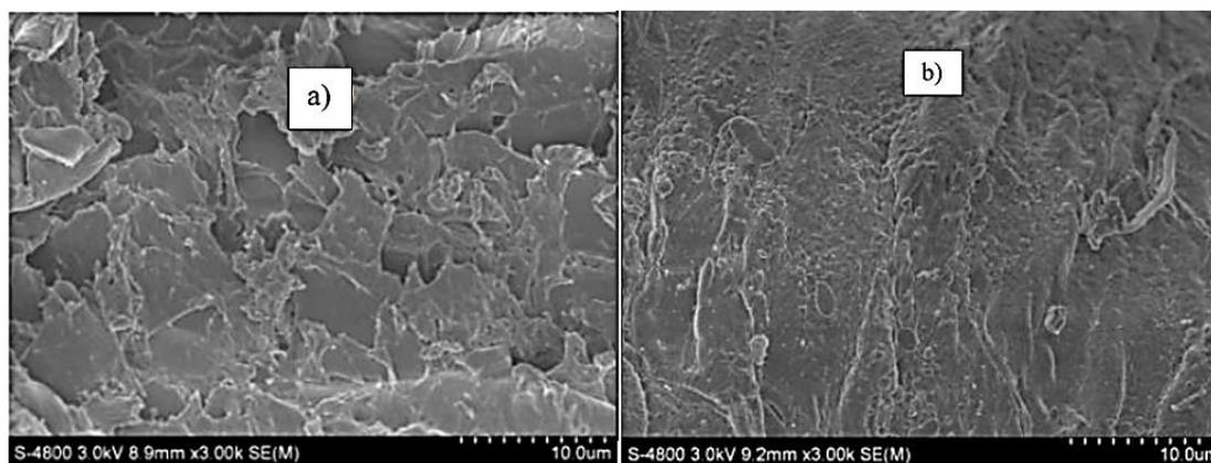
Figure 2.7: SEM Micrographs of Corncob Samples: (a) Untreated Corncobs (b) Pretreated Corncobs with 50 % v/v Ethanol (Varbanov et al., 2017)
