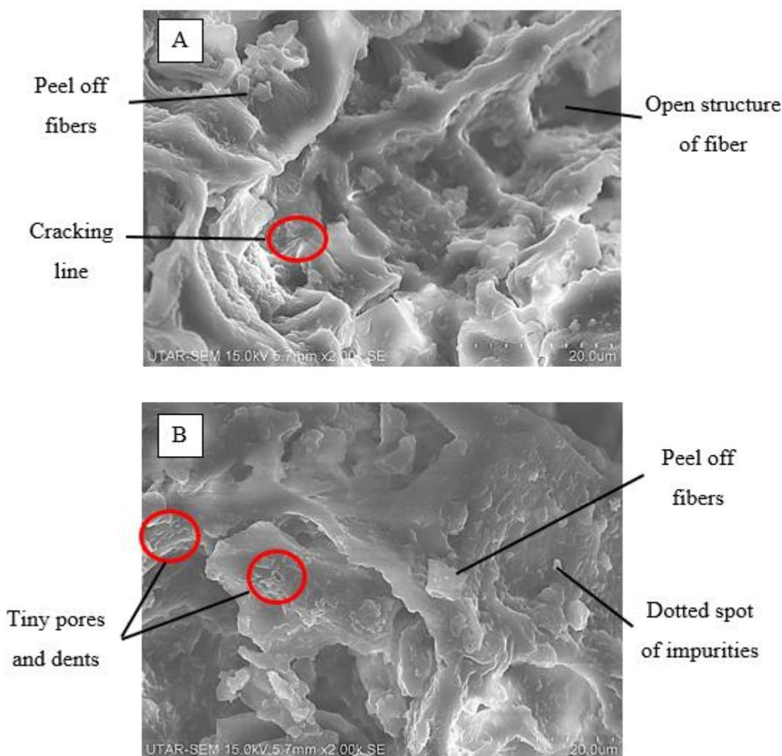
Figure 4.17: Surface Morphology of Treated Spent Coffee Grounds under 2000X Magnification at (A) 190 °C (B) 210 °C
