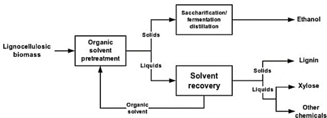
Figure 2.5: Flow Diagram of Organosolv Pretreatment of Lignocellulosic Biomass (Zhang, Pei and Wang, 2016)
