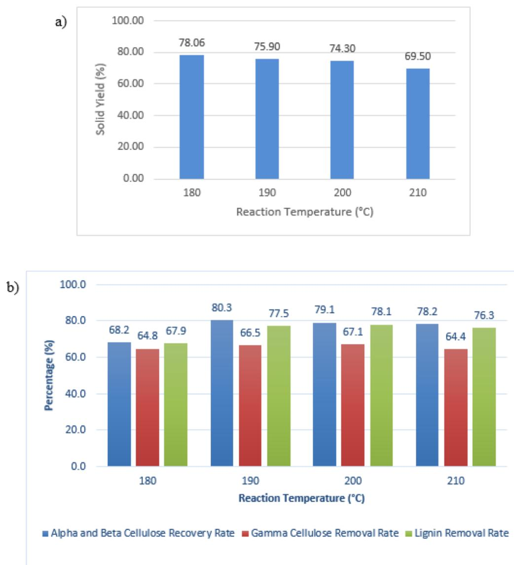
Figure 4.15: Pretreatment Performance under Solvent Loading of 12.5 % v/w with 1 % v/v acid for 60 Minutes But at Varying Reaction Temperature (a) Solid Yield after Organosolv Pretreatment (b) Alpha and Beta Cellulose Recovery Rate, Gamma Removal Rate and Lignin Removal Rate
