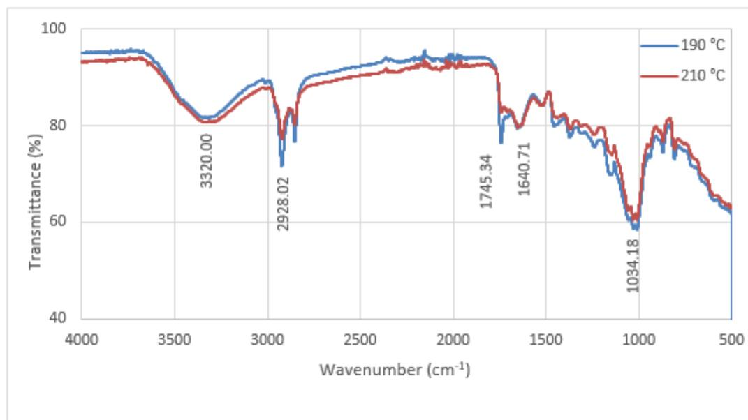
Figure 4.16: Comparison of FTIR Spectra of Treated Spent Coffee Grounds between Temperature of 190 °C and 210 °C
