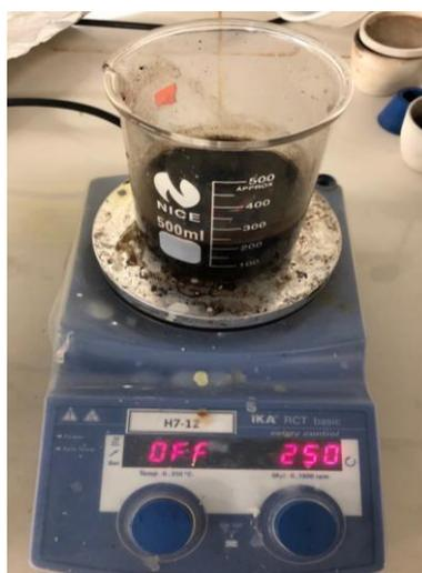
Figure 3.5: Stirring of Mixture at intervals of Washing Process at 250 rpm
