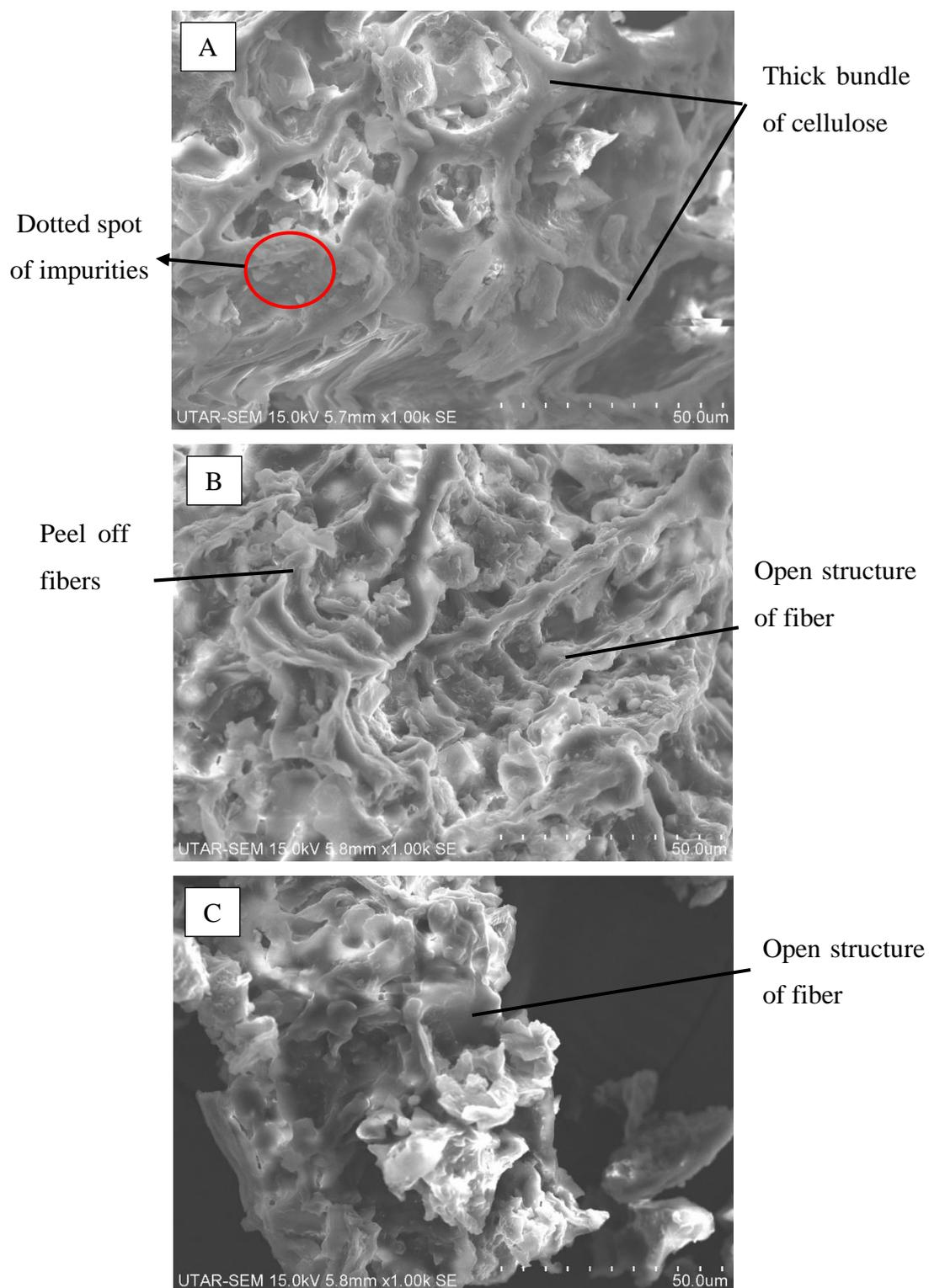
Figure 4.7: Surface Morphology of Raw and Treated Spent Coffee Grounds under Magnification of 1000 (A) Raw Spent Coffee Grounds (B) Treated Spent Coffee Grounds with Solvent Loading of 12.5 % v/w (C) Treated Spent Coffee Grounds with Solvent Loading of 17.5 % v/w
