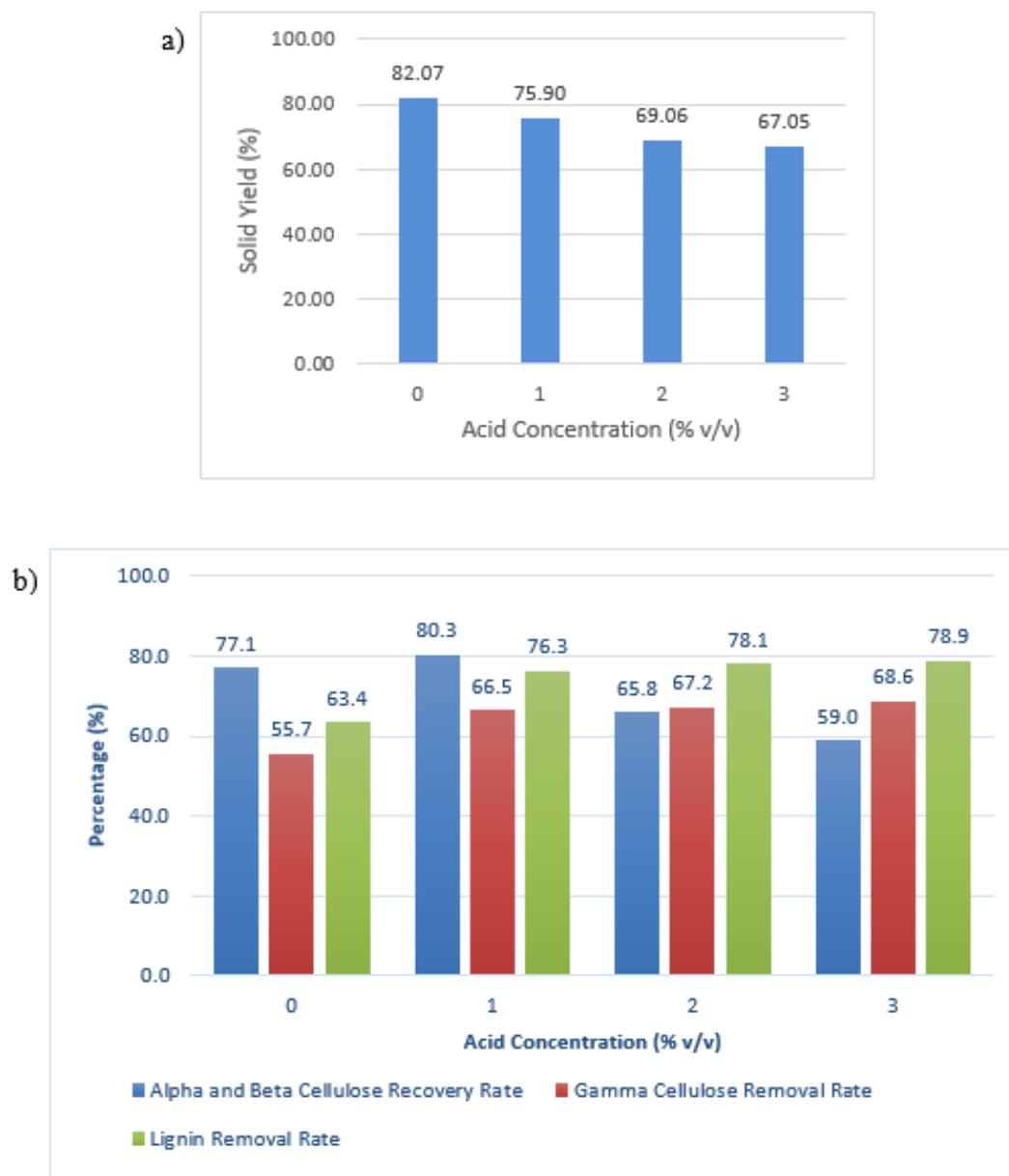
Figure 4.10: Pretreatment Performance at 190 °C for 60 Minutes under Solvent Loading of 12.5 % v/w But Varying Sulfuric Acid Concentration (a) Solid Yield after Organosolv Pretreatment (b) Alpha and Beta Cellulose Recovery Rate, Gamma Removal Rate and Lignin Removal Rate
