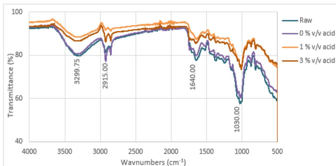
Figure 4.11: Comparison of FTIR Spectra between Raw and Treated Spent Coffee Grounds with Acid Concentration of 0, 1 and 3 % v/v
