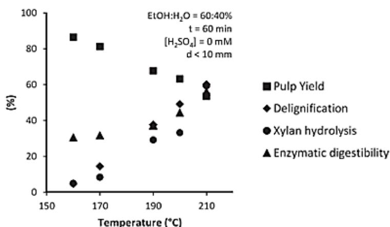
Figure 2.13: Organosolv Fractionation of Wheat Straw at Different Temperatures (Wildschut et al., 2013)
