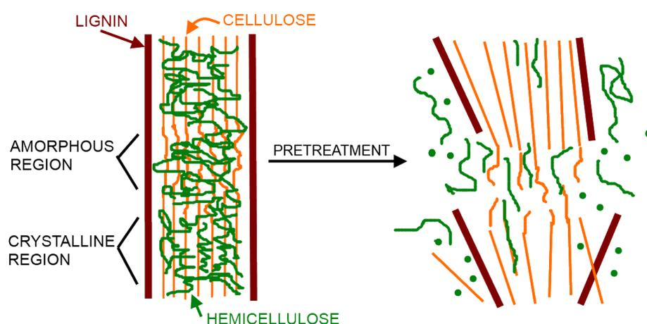
Figure 1.3: Impact of Pretreatment of Lignocellulosic Biomass (Zheng et al., 2014)
