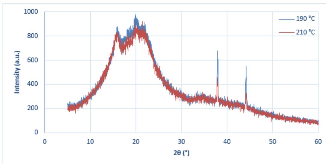
Figure 4.18: X-ray Diffractogram of Treated Spend Coffee Grounds at Temperature of 190 °C and 210 °C
