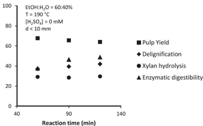
Figure 2.15: Organosolv Fractionation of Wheat Straw Against Reaction Time (Wildschut et al., 2013)
