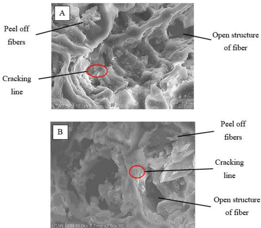
Figure 4.12: Surface Morphology of Treated Spent Coffee Grounds under 2000X Magnification (A) Acid Concentration of 1 % v/v (B) Acid Concentration of 3 % v/v
