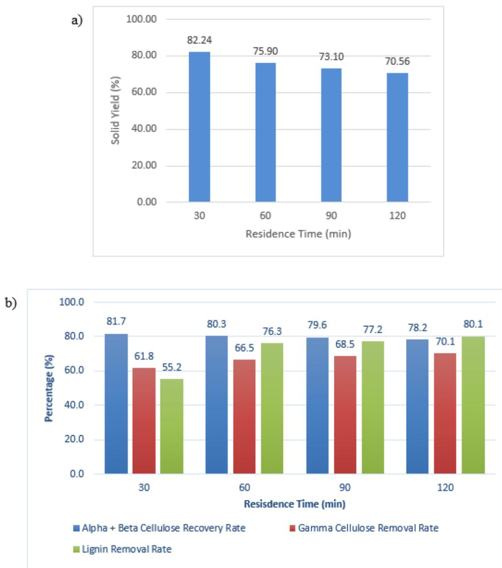
Figure 4.19: Pretreatment Performance at 190 °C under Solvent Loading of 12.5 % v/w with 1 % v/v acid But Varying Residence Time (a) Solid Yield after Organosolv Pretreatment (b) Alpha and Beta Cellulose Recovery Rate, Gamma Removal Rate and Lignin Removal Rate
