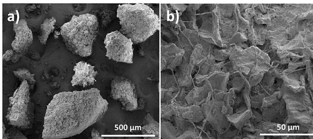
Figure 2.6: SEM Micrographs of Spent Coffee Grounds at Magnification of a) 200-Fold and b) 2000-Fold (Ballesteros, Teixeira and Mussatto, 2014)
