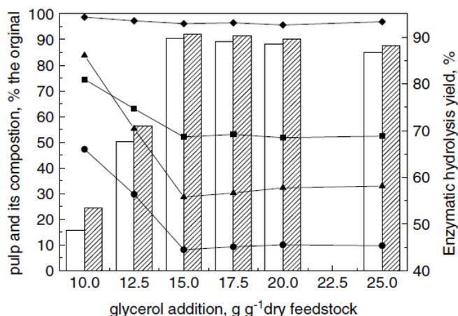
Figure 2.11: Effect of Varies Level of Glycerol Loading on Pretreatment of Wheat Straw at 240 °C for 4 hours. (Circle: Hemicellulose; Square: Pulp; Triangle: Lignin; Diamond: Cellulose; White Bar: 24 hours of Enzymatic Hydrolysis; Diagonal Hatched Bar: 48 hours of Enzymatic Hydrolysis) (Sun and Chen, 2007)
