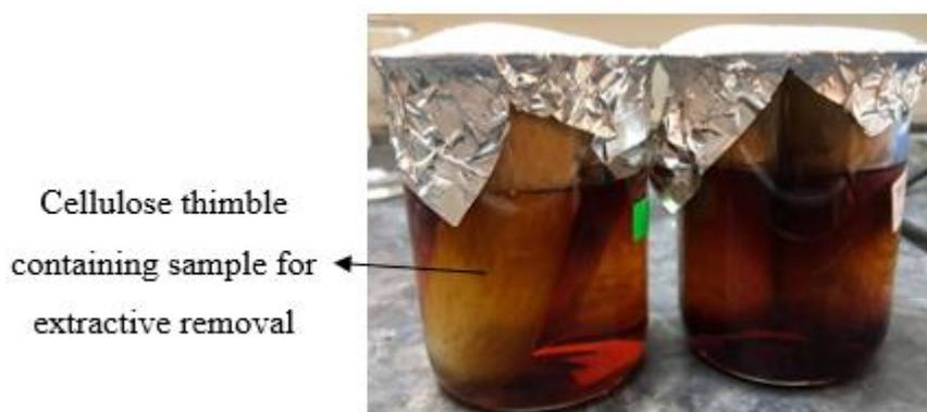
Figure 3.6: Soaking of Pretreated SCG in Solvent Mixture for 24 hours
