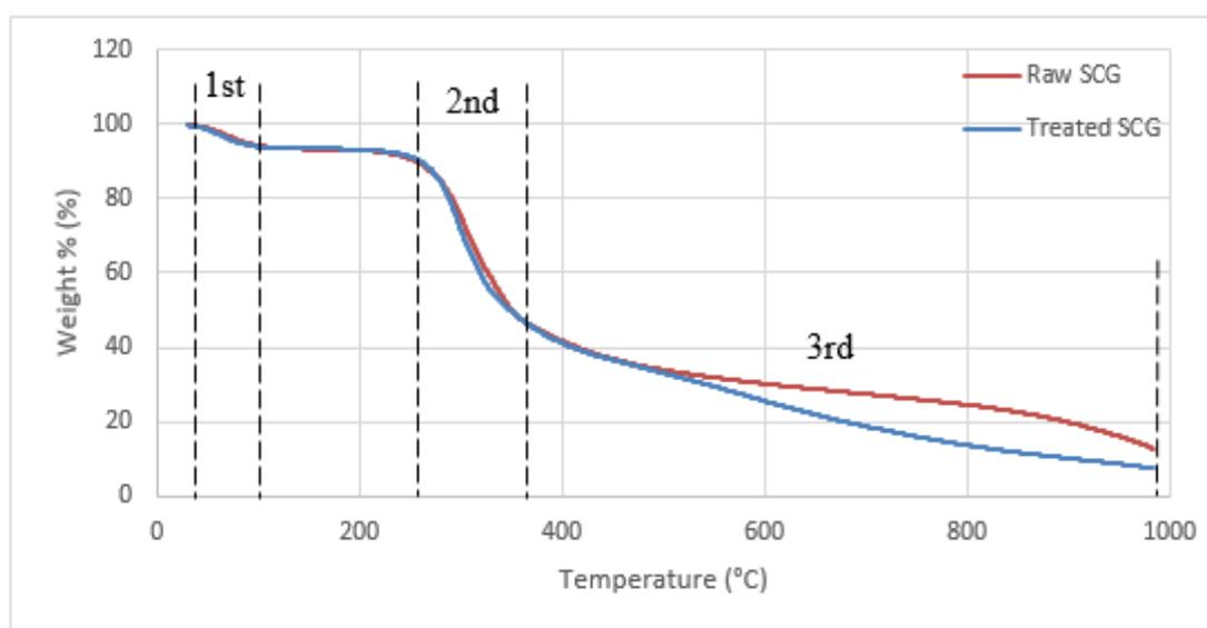
Figure 4.9: Comparison of TGA Curve between Raw and Treated Spent Coffee Grounds with Solvent Loading of 12.5 % v/w
