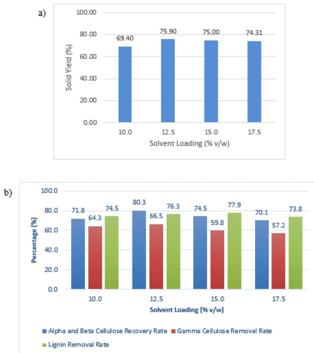
Figure 4.5: Pretreatment Performance at 190 °C for 60 Minutes Using 1 % v/v Acid But Varying Solvent Loading (a) Solid Yield after Organosolv Pretreatment (b) Alpha and Beta Cellulose Recovery Rate, Gamma Removal Rate and Lignin Removal Rate
