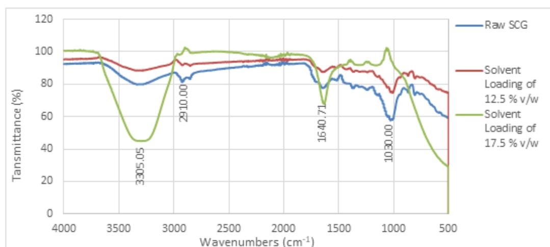
Figure 4.6: Comparison of FTIR Spectra between Raw and Treated Spent Coffee Grounds with Solvent Loading of 12.5 % v/w and 17.5 % v/w
