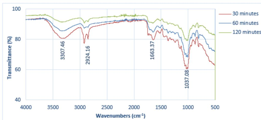
Figure 4.20: Comparison of FTIR Spectra for Treated Spent Coffee Grounds at Residence Time of 30, 60 and 120 minutes
