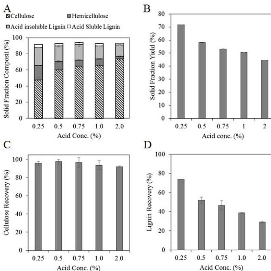
Figure 2.12: Effect of Sulfuric Acid Concentration on: A) Solid Fraction Composition, B) Solid Fraction Yield, C) Cellulose Recovery and D) Lignin Recovery (Teramura et al., 2018)
