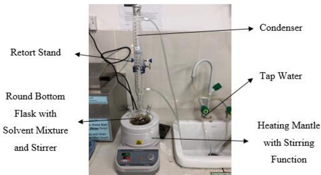
Figure 3.3: Experimental Set Up for Organosolv Pretreatment
