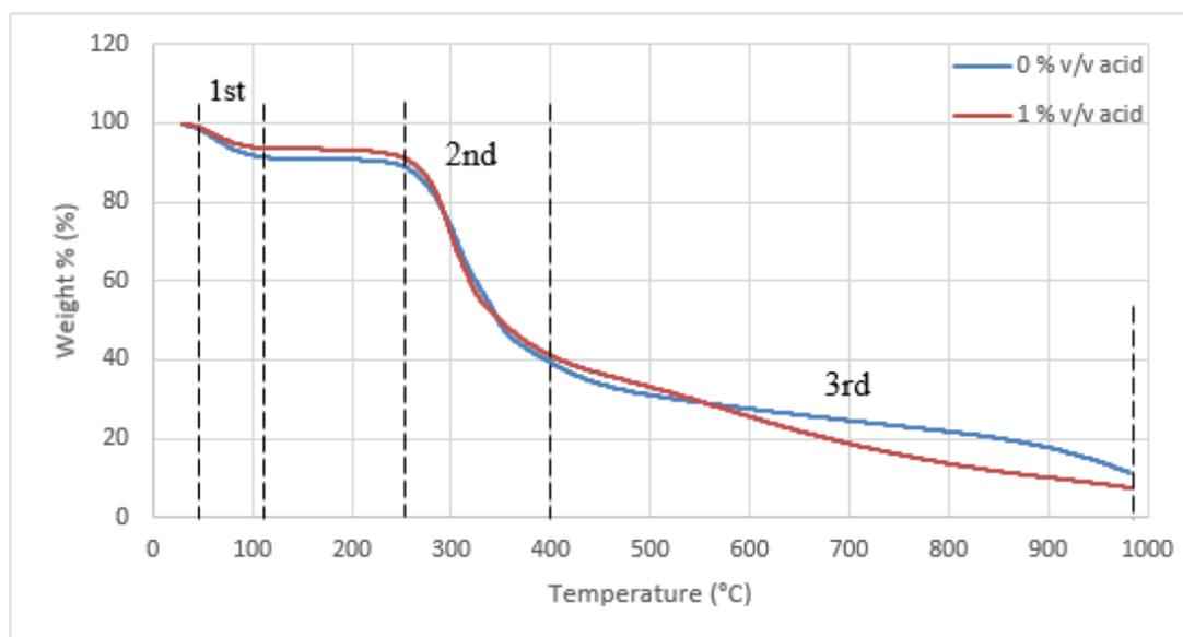
Figure 4.14: Comparison of TGA Curve between Pretreated Spend Coffee Grounds with 1 % v/v of Acid and Without Catalyst
