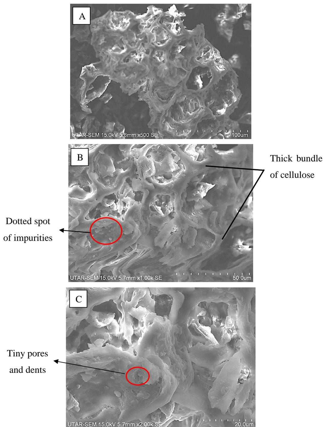
Figure 4.1: Surface Morphology of Raw Spent Coffee Grounds under Magnification of (A) 500X (B) 1000X and (C) 2000X
