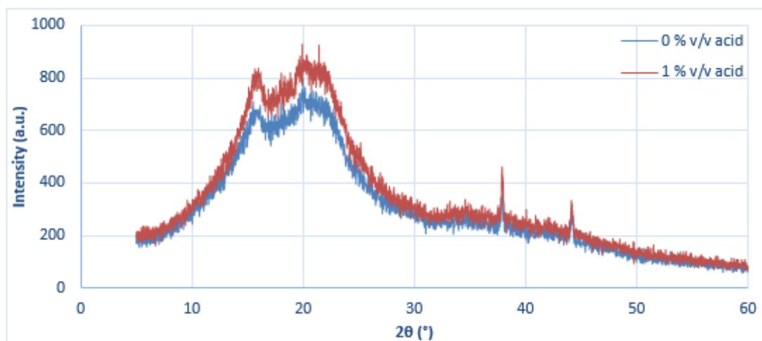
Figure 4.13: X-ray Diffractogram of Pretreated Spend Coffee Grounds with 1 % v/v of Acid and Without Catalyst
