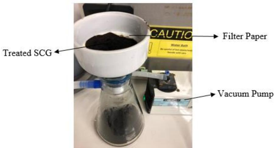
Figure 3.4: Filtration Step using Vacuum Pump
