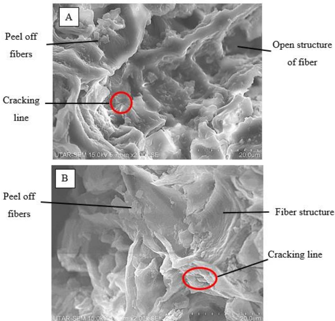
Figure 4.21: Surface Morphology of Treated Spent Coffee Grounds under 2000X Magnification at (A) 60 minutes (B) 120 minutes
