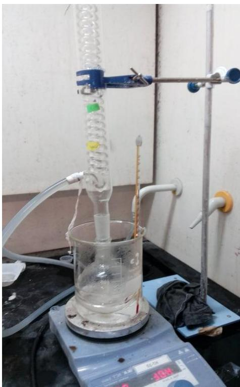
Figure 4.3: Determination of Cellulose Content by Acid Hydrolysis Using Dilute Hydrochloric Acid Solution for 2 Hours at 50 °C
