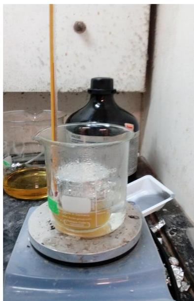
Figure 4.1: Determination of Holocellulose Content Using Mixture of Glacial Acetic Acid and Sodium Chlorite Solution for 90 Minutes at 90 °C
