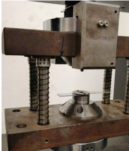
Figure 3.14 Setup of clinching process
