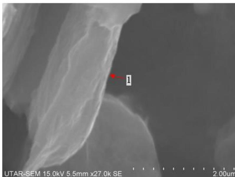
Figure 4.6: Graphene SEM Image at the Magnification of 27 000x
