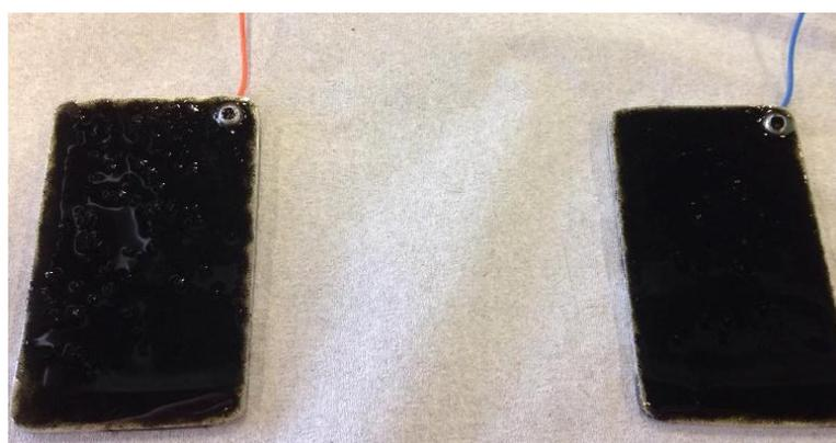
Figure 3.16: Aluminium Plates with a Layer of  $FeCl_3 - FLG$
