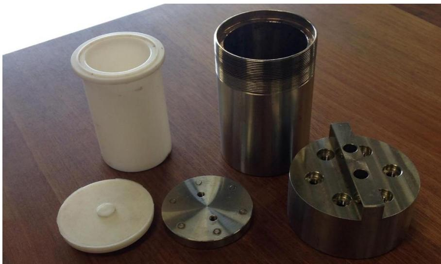
Figure 3.8: 50 mL Stainless Steel Autoclave
