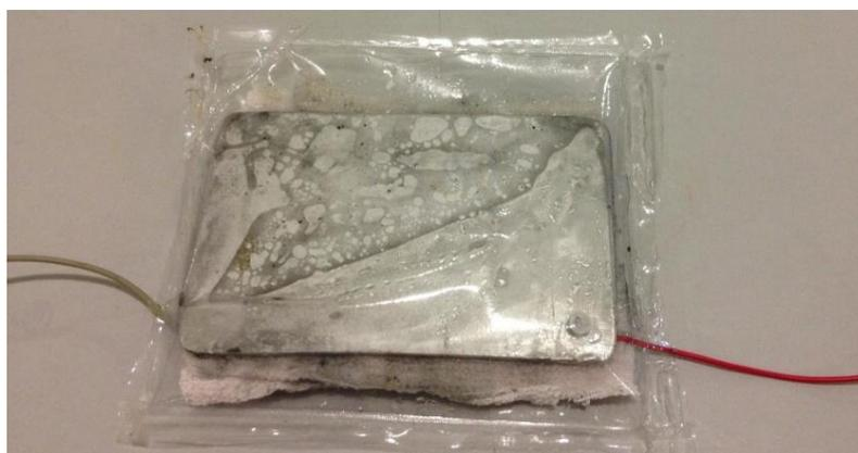
Figure 3.17: Sealed  $FeCl_3 - FLG$  Supercapacitor
