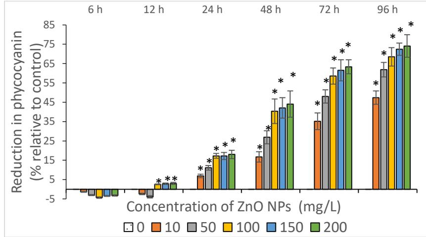
**Figure 4.17: Percentage of loss in phycocyanin content of *S. platensis* upon treatment with ZnO NPs.**
