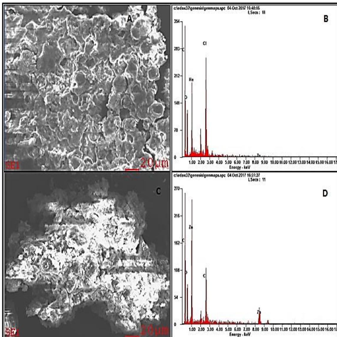
**Figure 4.4:** Scanning electron microscopic micrograph of *H. pluvialis* biomass (A) with EDX spectrum (B). Scanning electron microscopic micrograph of *H. pluvialis* biomass exposed to 200 mg/L of ZnO NPs at 96 h (C) with EDX spectrum (D).
