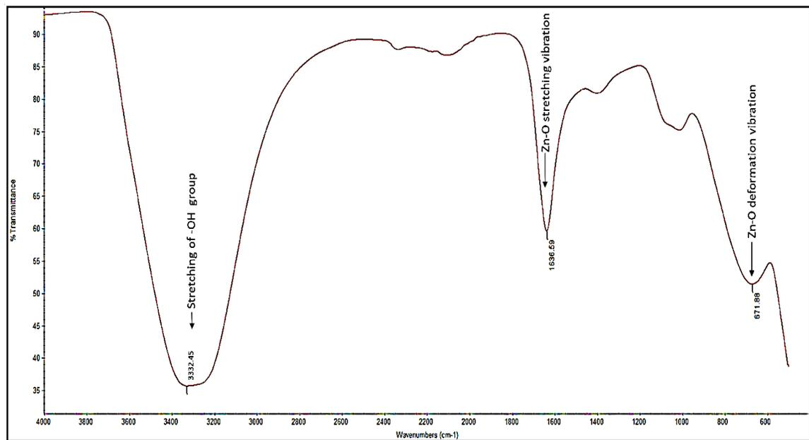
**Figure 4.2: FTIR spectrum of zinc oxide nanoparticles powder**
