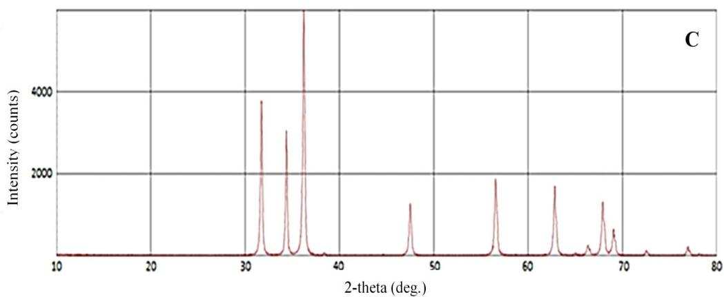
**Figure 4.1: Scanning electron microscopy image (A), X ray energy dispersive spectroscopy spectrum (B) and X-ray diffractometer spectrum (C) of ZnO NPs.**
