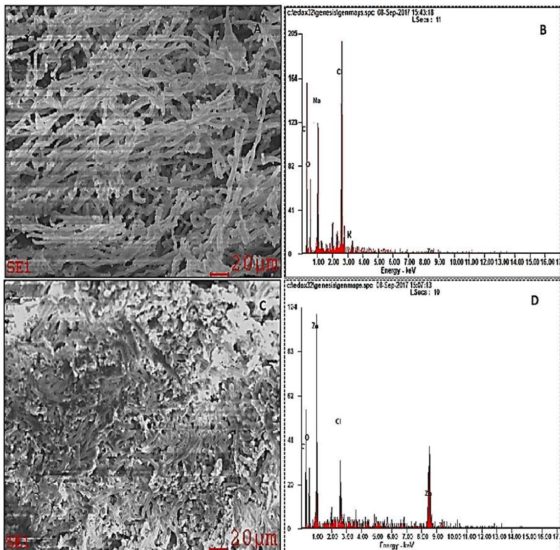
**Figure 4.3:** Scanning electron microscopic micrograph of *S. platensis* biomass (A) with EDX spectrum (B). Scanning electron microscopic micrograph of *S. platensis* biomass exposed to 200 mg/L of ZnO NPs at 96 h (C) with EDX spectrum (D).
