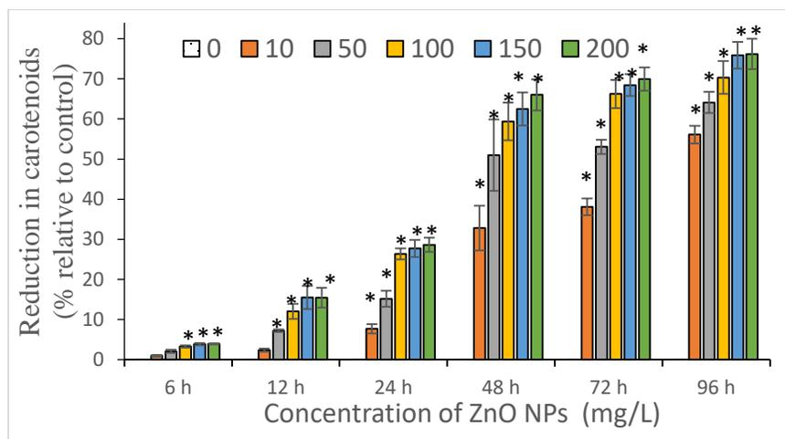
**Figure 4.15: Percentage of loss in carotenoids of *S. platensis* upon treatment with ZnO NPs.**
