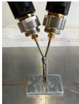
Figure 2.15: Experimental setup for measuring the input impedance.
