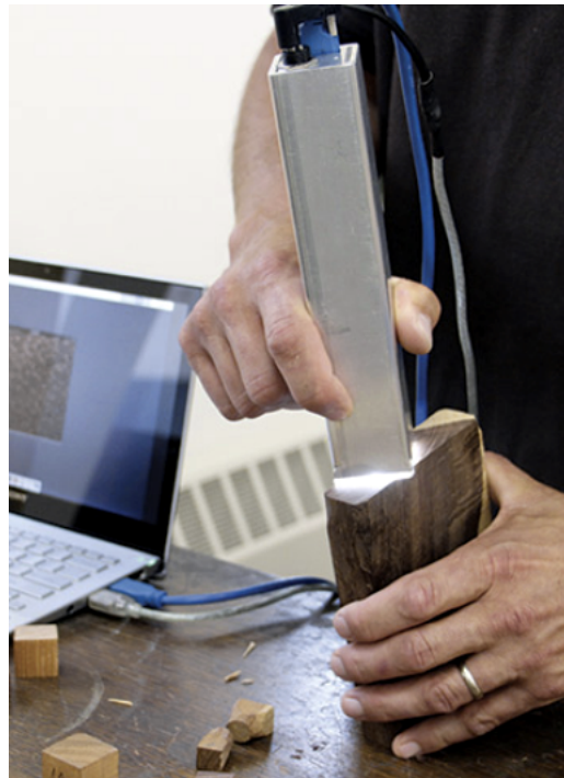
FIGURE 2.4: A demonstration of Xylotron device on wood identification
