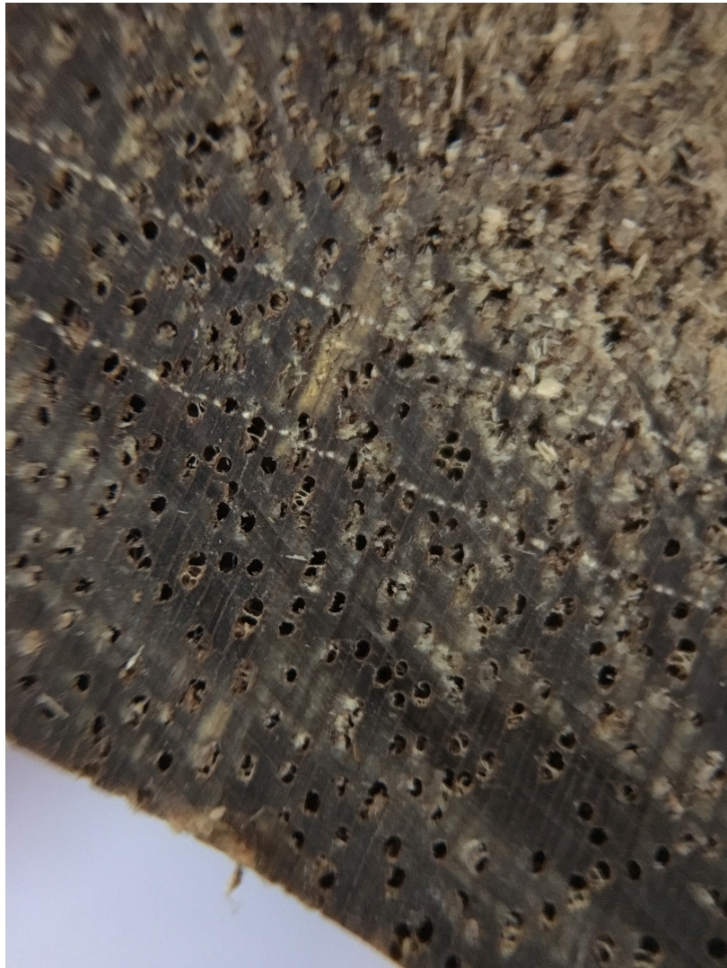
FIGURE 2.1: Example of textures observed at macroscopic level on transverse cross section of Dark Red Meranti captured using smart-phone with macro-lens.
