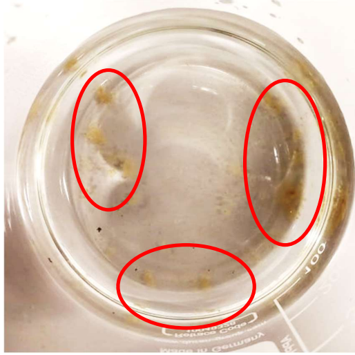
Figure 5.7: Detached Activated Sludge found in the Effluent on Day 21.
