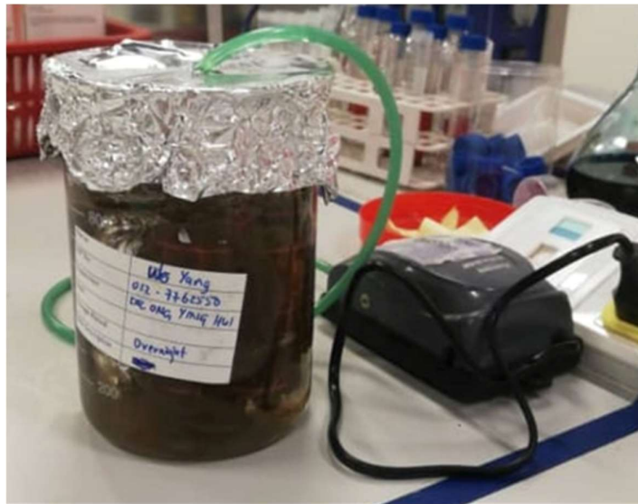
Figure 3.4: Cultivation of Activated Sludge on Sponge Media.
