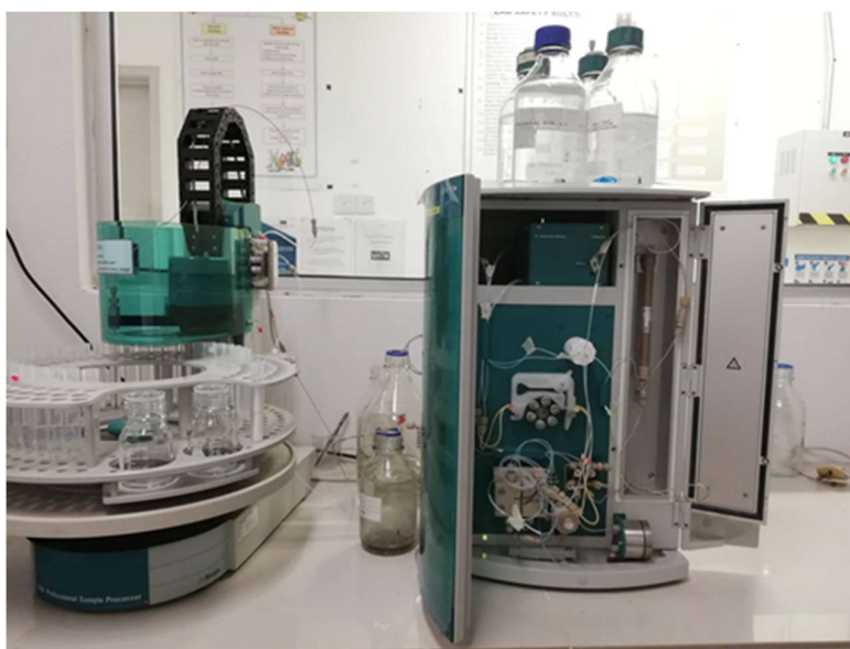
Figure 3.7: Ion Chromatography for Phosphate Test.
