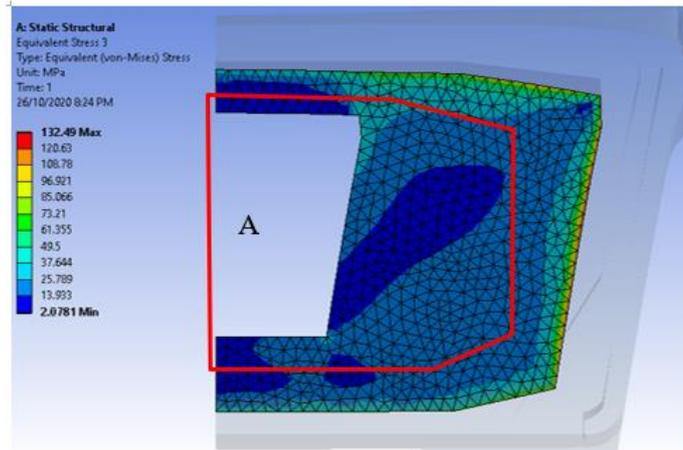
Figure 4.6: Area that Affected by Stress Effect from Transverse Direction
