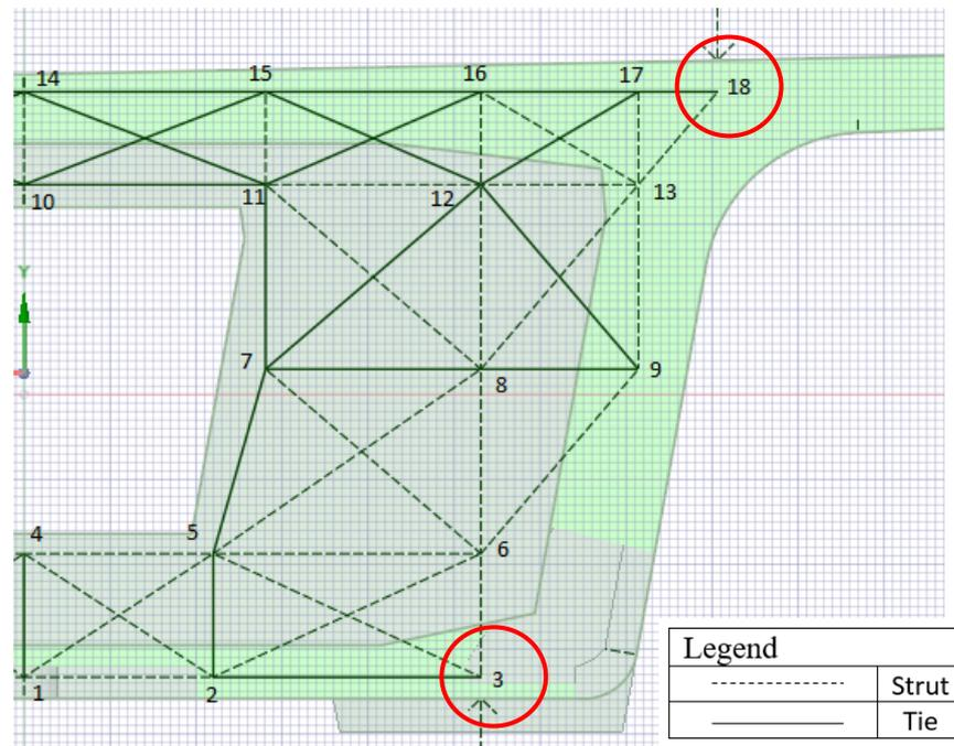
Figure 4.9: Proposed STM Connections before Optimisation Process
