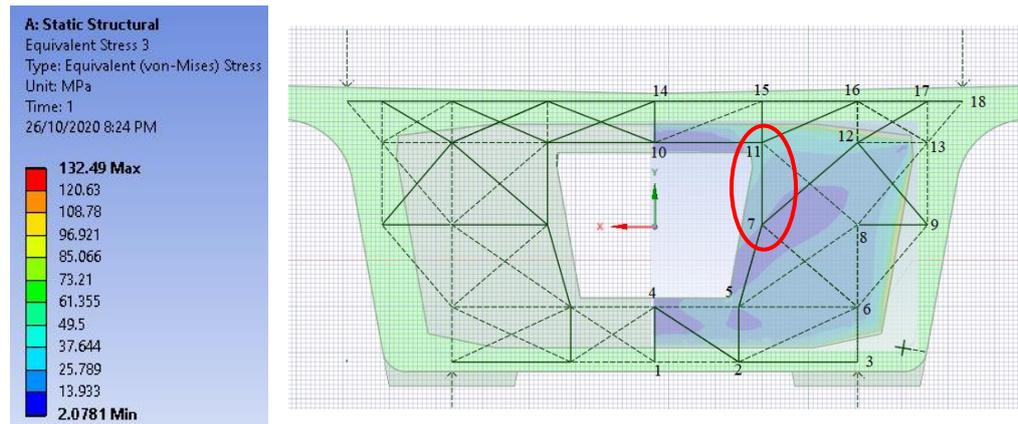
Figure 4.12: Combination of STM and Stress Distribution Result from ANSYS
