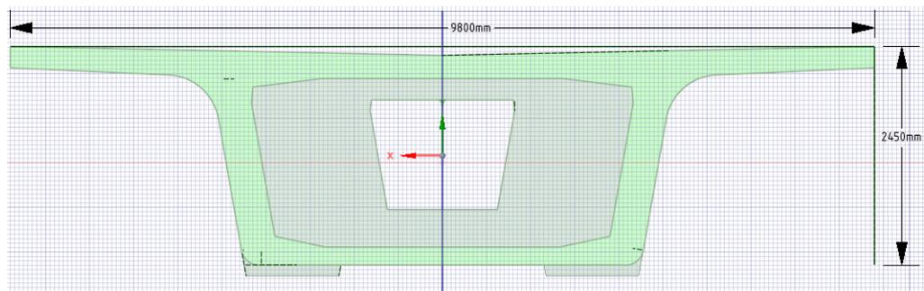
Figure 4.1: Layout of Full Box Girder
