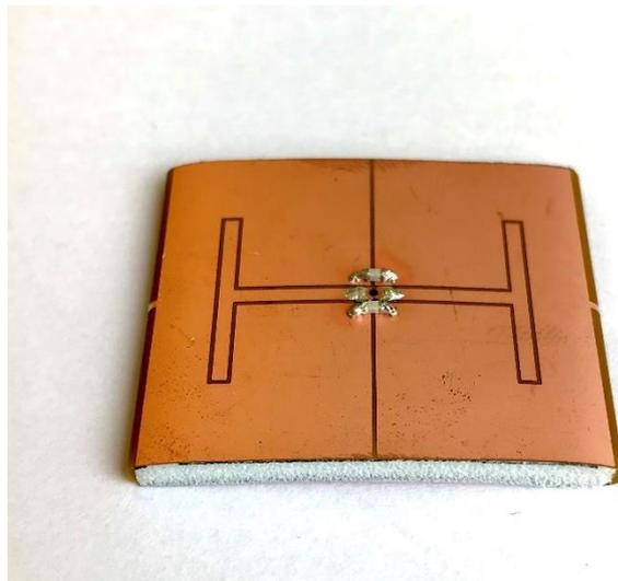
**Figure 4.1:** (a) Antenna configuration. (b) Prototype of proposed tag antenna.
