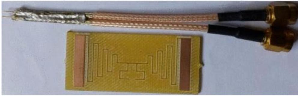
**Figure 2.7:** Fabricated prototype of a meandered dipole.
