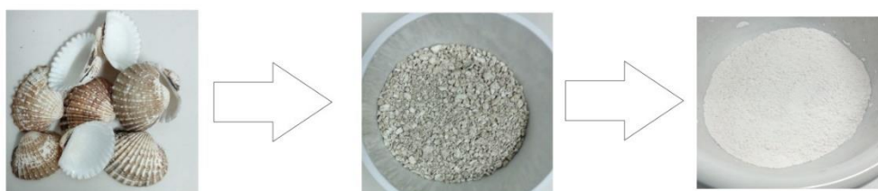
Figure 3.2: Catalyst preparation from cockle shell to CaO catalyst prepared via calcination treatment and then nano CaO catalyst prepared via thermal hydration-dehydration treatment
