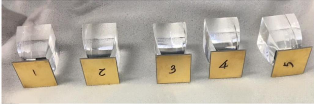
Figure 3.13: Five unit of CCPC-CPV assembly modules used for indoor measurement.
