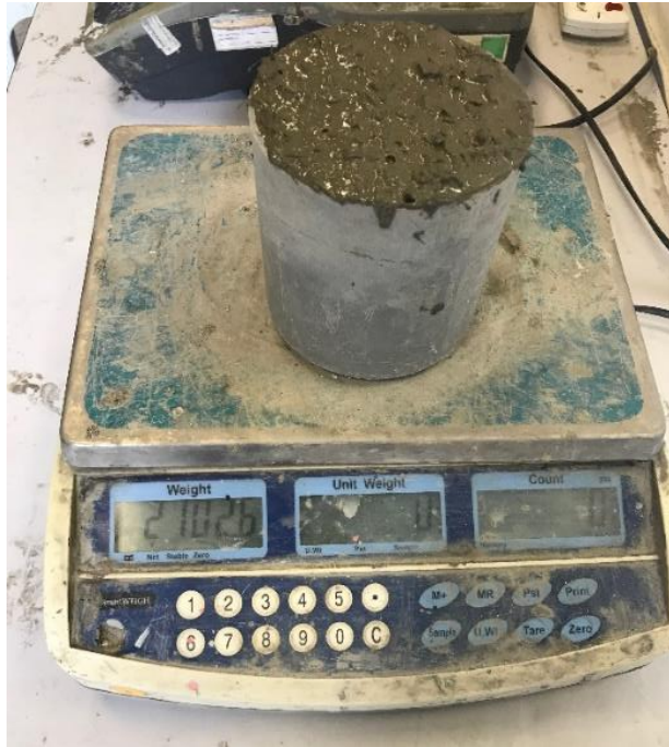
Figure 3.6: Measurement of Fresh Density
