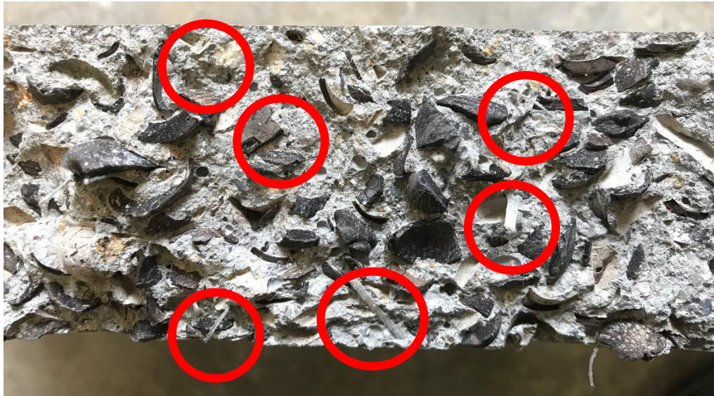
Figure 4.24: Cross-Section of OPSLWC-HYB-0.4% with Randomly Distributed Fibres
