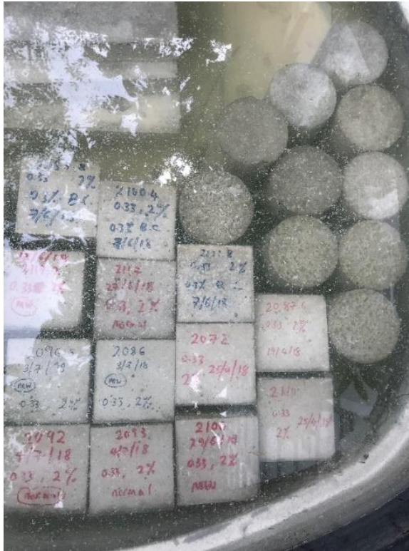
Figure 3.5: Specimens in the Water Tank for curing
