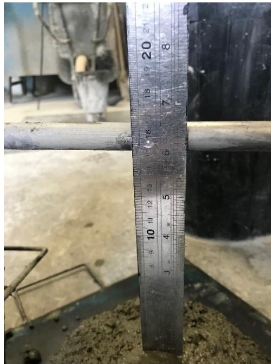
Figure 3.7: Measurement of Slump Value.
