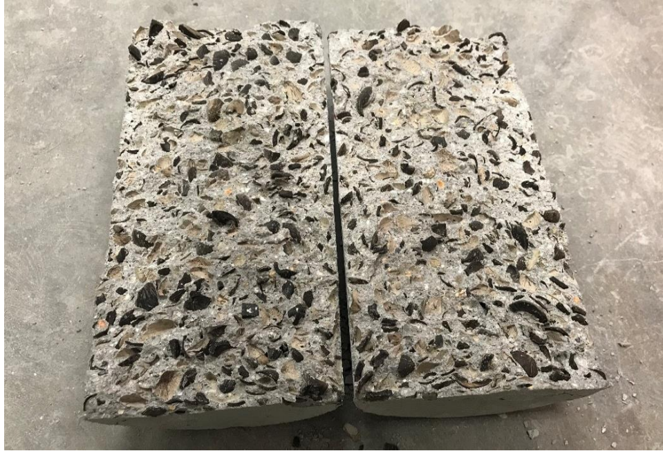
Figure 4.14: Failure Mode of OPSLWC-CTR-0% after First Loading
