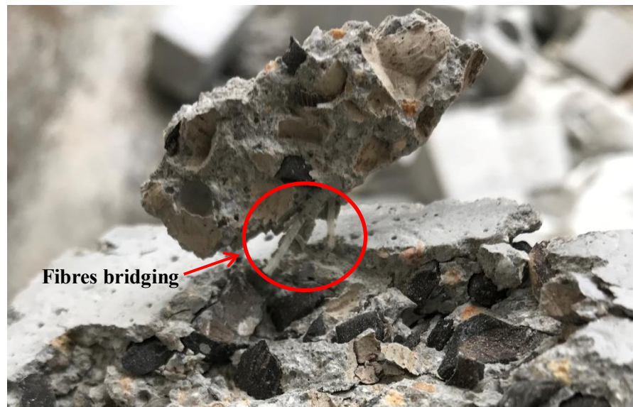
Figure 4.11: Linking Bridge between Fibres and Cement Matrices
