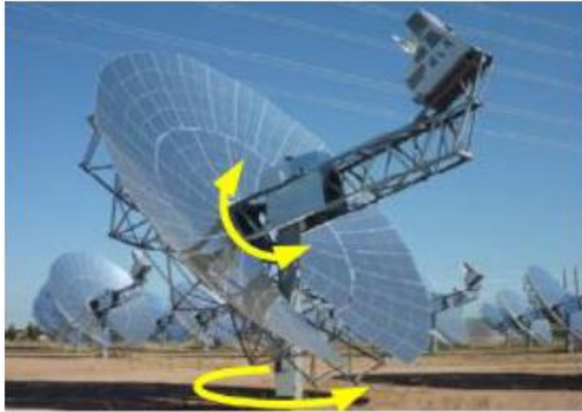
Figure 2.5 Applications of 2 axis sun-tracking (ST) system for solar thermal dish (Rockwell Automation, 2011)
