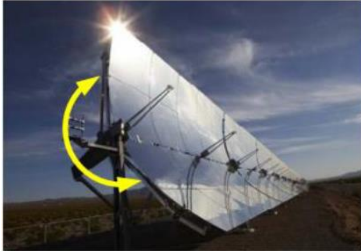
Figure 2.3: Applications of 1 axis sun-tracking (ST) system for solar thermal parabolic trough (Rockwell Automation, 2011)
