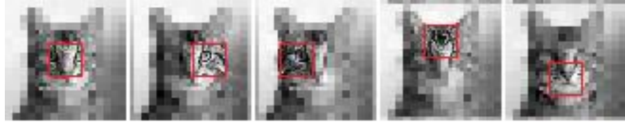
Figure 4.12: (From left to right) A demonstration of programming the fovea to prioritize different regions of “cat”. Notice that except for the fovea, the rest of the regions of the image is in low-resolution.
