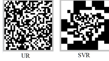
Figure 3.5: Examples of an UR CPA sensing pattern and an SVR CPA sensing pattern. The SVR sensing pattern shown here was formed by mapping the UR sensing pattern onto an SVR grid via the transformation matrix \tau . The UR sensing pattern is made up of 1024 regular sized pixels and the SVR sensing pattern is made up of 363 cells. Both patterns are of the same size 32 \times 32 .
