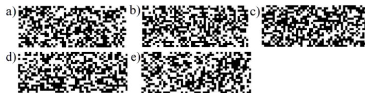
Figure 3.3: Five CPA sensing matrices of size 20 \times 50 generated with z_0 = (a) 0.19 (b) 0.39 (c) 0.59 (d) 0.79 (e) 0.99. The white squares represent the entries +1 while the black squares represent the entries -1.
