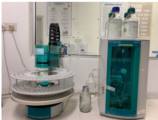
Figure 3.4: Ion Chromatography, Metrohm 861 Advanced Compact IC
