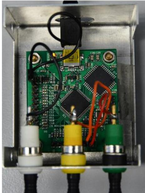
Figure 4.1 Fabricated EEG acquisition unit housed in an aluminium case with 3 terminals for signal, ground and reference.
