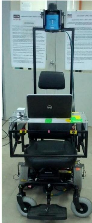
Figure 4.6 Prototype autonomous wheelchair with PC, BCI acquisition unit, NAV350 navigation laser range finder and ultrasonic sensors
