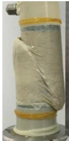
Figure 2.15: Failure patterns for heavily treated sand in undrained compression test (Cui et al., 2017)
