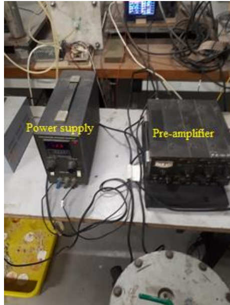
Figure 3.37: Power supply and pre-amplifier
