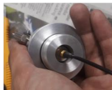
Figure 3.34: Procedure of installing AE transducer into base pedestal
