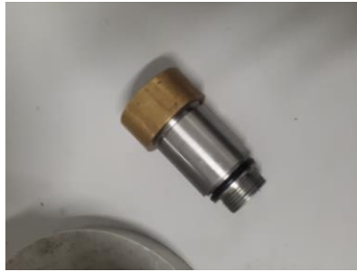
(a) Photo of loading shaft
