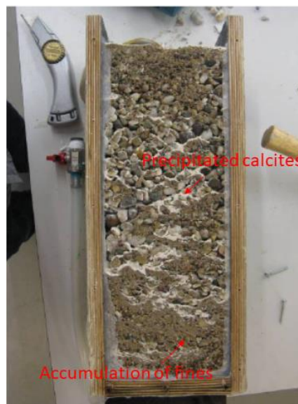
Figure 2.23: Heterogeneous calcite distribution (Van Paassen, 2011)
