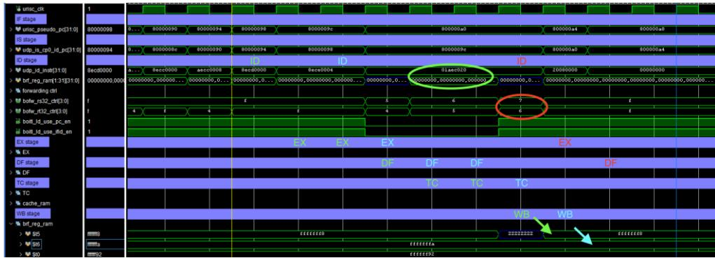
Figure 6-22: Simulation Result I for D-Cache Load-Use Test.
