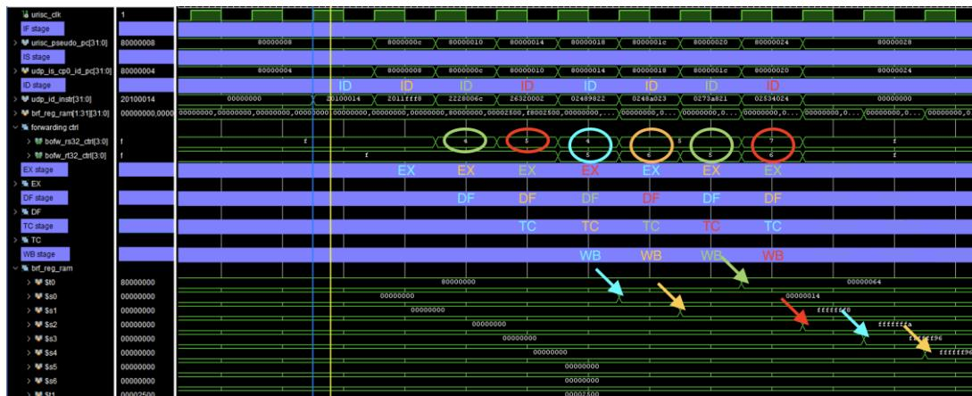
Figure 6-13: Simulation Result I for ID.rs and ID.rt Route Forwarding Test.
