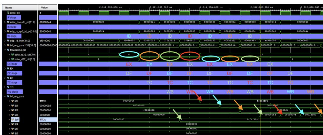
Figure 6-14: Simulation Result II for ID.rs and ID.rt Route Forwarding Test.
