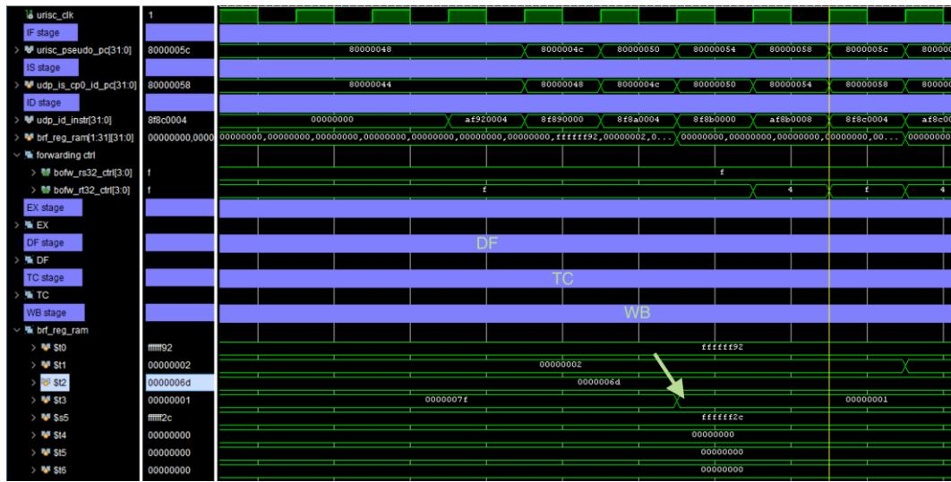
Figure 6-15: Simulation Result III for ID.rs and ID.rt Route Forwarding Test.
