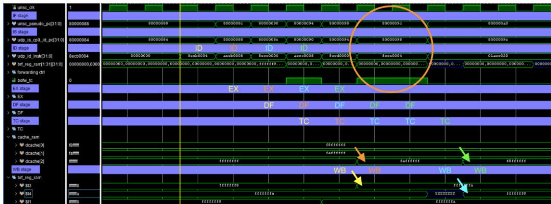
Figure 6-21: Simulation Result for D-Cache Load-Store Test.
