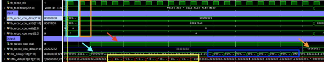
Figure 6-7: Simulation Result for Test 7: Write Hit followed by Read Miss FIFO Miss.
