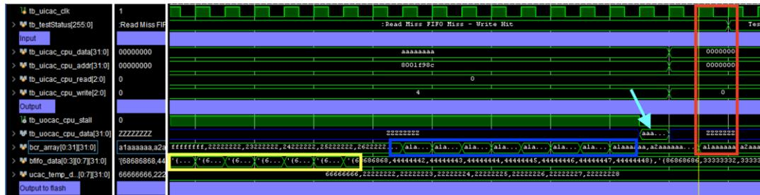
Figure 6-12: Simulation Result II for Test 11: Read Miss FIFO Miss followed by Write Hit.
