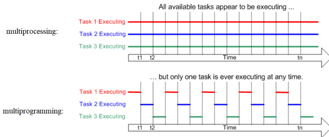
Figure 3.2.1 Multiprocessing and multiprogramming
