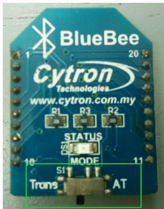
Figure 5.3 Green box show the Cytron Bluetooth module change to Trans mode.
