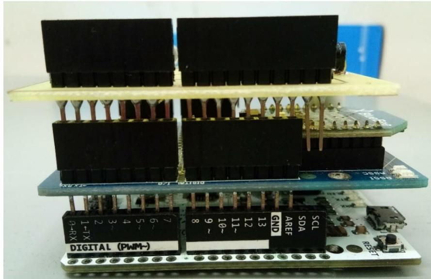
Figure 5.6 Side view after mounted created infrared board on the Cytron XBee Shield.
