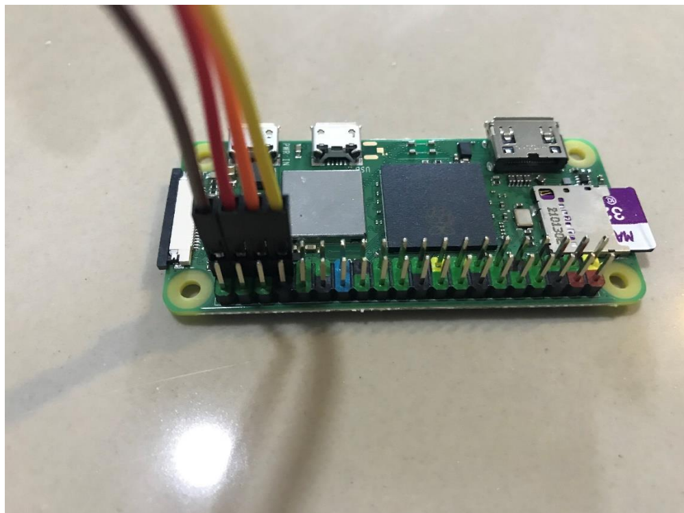
Figure 5.1.3b Wiring of RPi Zero W
