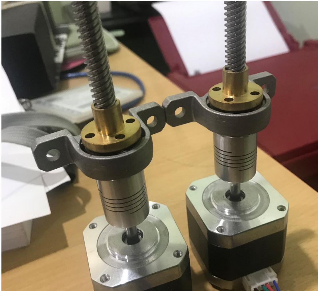
Figure 5.1.2 Motors connected to lead screw with coupling shaft
